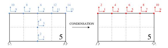
Figure 4.10: Condensation of the fifth substructure
