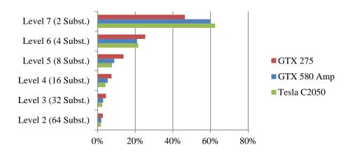
Figure 4.22: The ratio of dense condensation time values to total dense condensation time
