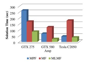
Figure 4.24: The shortest solution times obtained from the solution of 160×160 meshed structure with the three methods
