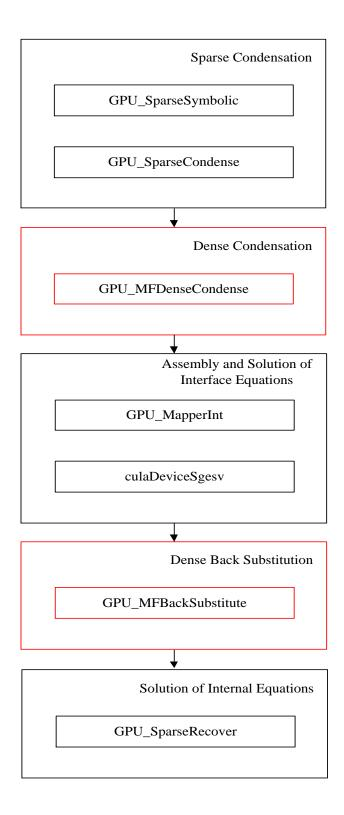
Figure 4.13: Subroutines used for GPU implementation of multifrontal algorithm
