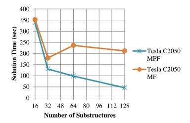
Figure 4.20: Solution time of the structure with 160×160 elements with Tesla C2050
