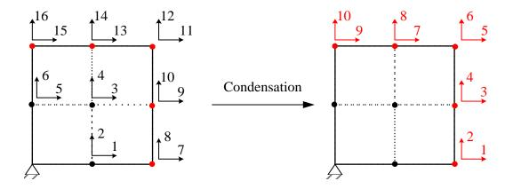
Figure 3.7: Condensation of the first substructure
