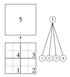
Figure 3.3: Assembly tree with four substructures
