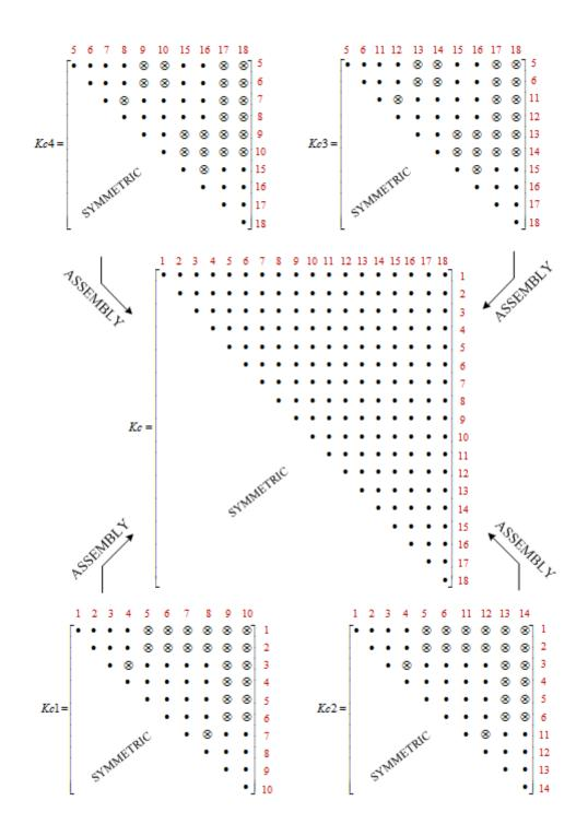
Figure 3.11: Assembly of Interface Matrix
