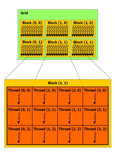
Figure 2.6: Organization of Grid and Thread Blocks [18]
