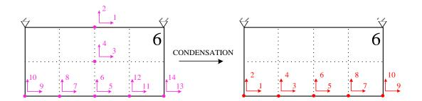
Figure 4.11: Condensation of the sixth substructure
