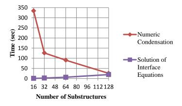
Figure 3.17: The sparse condensation time and solution time of the interface equations for 160×160 structure
