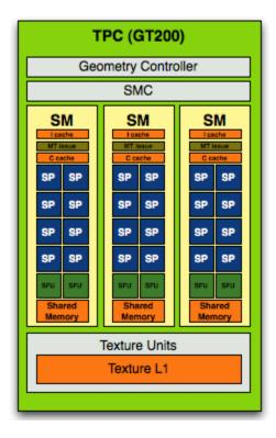
Figure 2.3: Architecture of a texture/processor cluster (TPC) [50]
