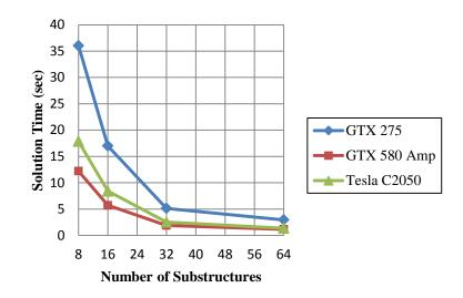
Figure 3.14: Solution time values obtained from the solution of the structure with 50×50 elements
