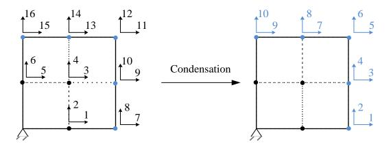
Figure 4.7: Condensation of the first substructure
