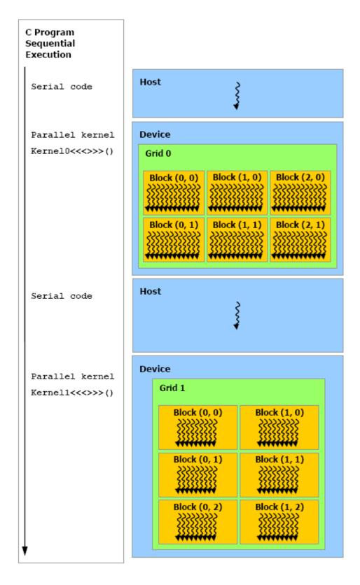
Figure 2.9: Use of both CPU and GPU [18]
