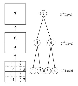
Figure 4.2: Assembly tree for a 4×4 square mesh with three levels
