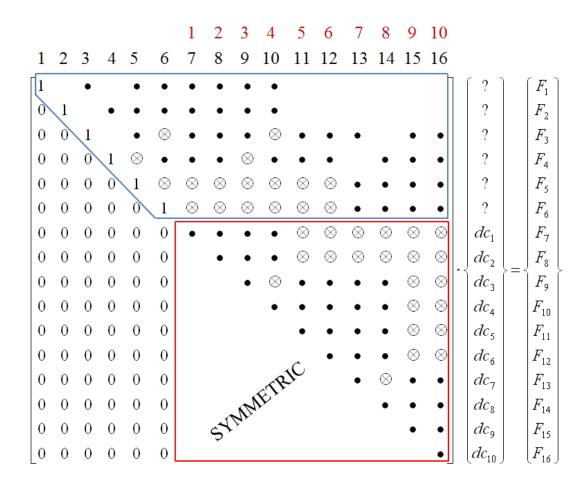
Figure 3.12: System of Equations for Substructure 1
