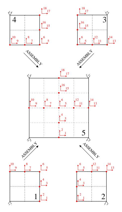
Figure 3.10: Assembly of Substructures
