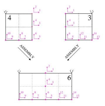
Figure 4.9: Assembly of the last two substructures
