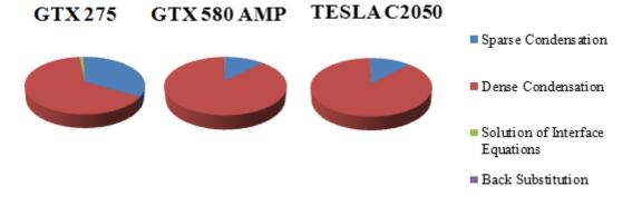
Figure 4.21: The effect of solution steps to the solution time of structure with 160×160 elements with 128 substructures
