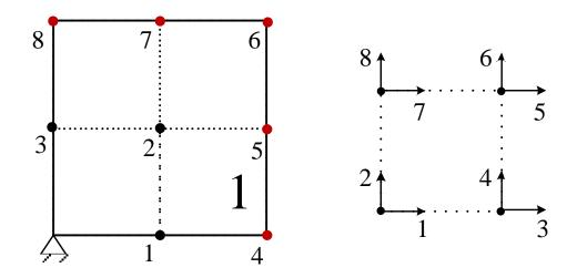
Figure 3.6: Substructure 1 and a bilinear 4-node membrane element
