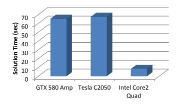
Figure 4.25: The solution time of the 200×200 structure with different architectures.
