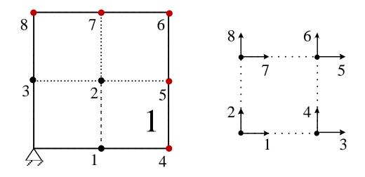
Figure 4.6: Substructure 1 and a bilinear 4-node membrane element
