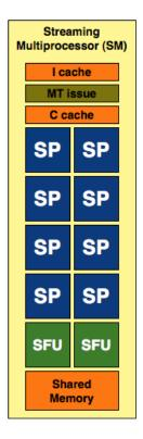
Figure 2.2: Architecture of a streaming multiprocessor (SM) [50]
