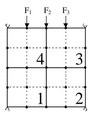
Figure 4.5: Example structure with 4×4 mesh
