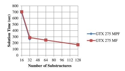
Figure 4.18: Solution time of the structure with 160×160 elements with GTX 275
