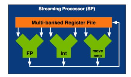
Figure 2.1: Architecture of a streaming processor (SP) [50]
