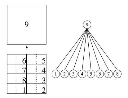
Figure 3.4: Assembly tree with eight substructures
