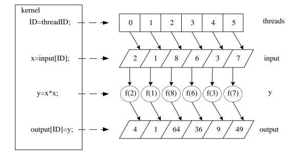
Figure 2.5: Execution of an example kernel by multiple threads
