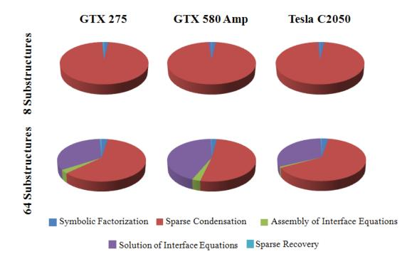
Figure 3.16: The effect of solution steps to the solution time of structure with 50×50 elements with 8 and 64 substructures
