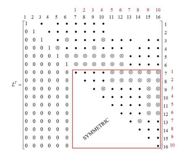
Figure 3.9: Transpose of the unit lower triangular matrix
