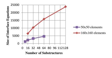
Figure 3.18: Sizes of interface equations of both structures for various numbers of substructures
