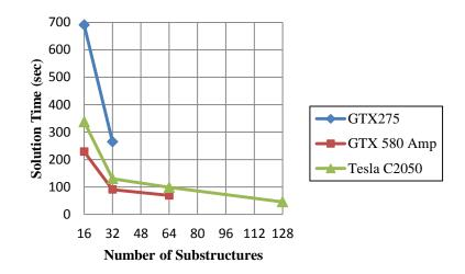
Figure 3.15: Solution time values obtained from the solution of the structure with 160×160 elements
