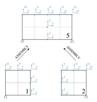
Figure 4.8: Assembly of the first two substructures
