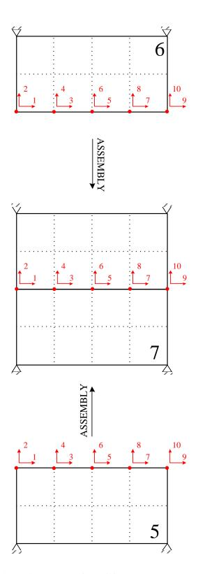
Figure 4.12: Assembly of the fifth and sixth substructures
