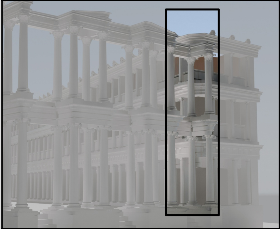
Figure 34 - NW corner of South Portico with collided blocks on 3D model of the Sebasteion (reliefs are not included in this render)
