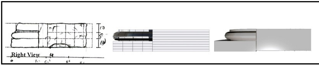
Figure 29 - Three steps of a Doric Column Base of the model. From left to right; Field Drawing, Wireframe Model and the Final Product
