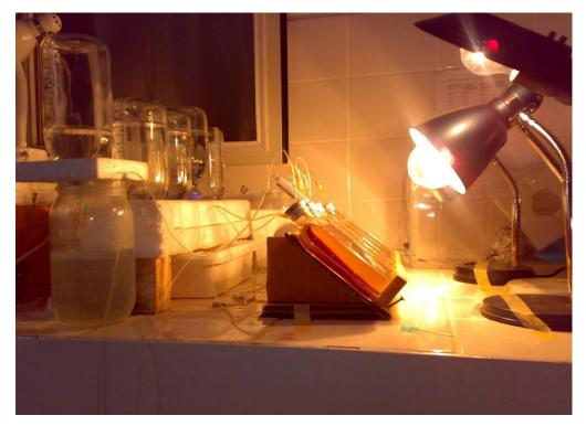
Figure 2.1 Experiment setup for hydrogen production by immobilized *R. capsulatus* in 250 ml cell culture bottles
