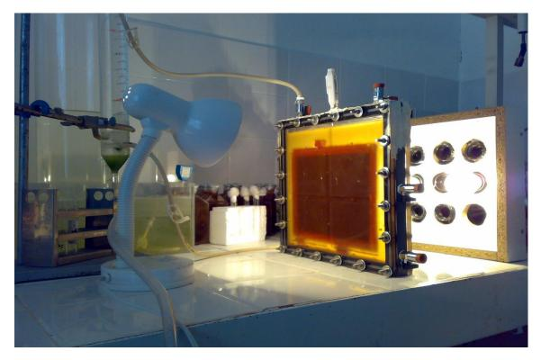
Figure 2.5 Experiment setup for hydrogen production by immobilized *R. capsulatus* panel photobioreactor
