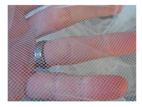
Figure 4.59 A photograph of a piece of Tulle fabric used for supporting and reinforcement of agar for bacterial immobilization in panel reactor
