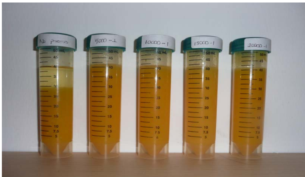
Figure 3.9 Stability of orange juices after 14 days storage at 4 °C after squeezed and microfluidized
