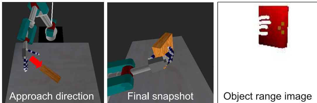
Figure 9.2: The execution of power-grasp behavior and the final object range image. The arrow shows the corresponding approach direction ( \alpha ).
