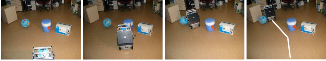
Figure 6.8: The course of the real robot trained with curiosity-driven scheme. The initial position of the robot is shown in the left-most figure. The robot first goes forward, then turns left since trash-bin does not afford traversability. Third snapshot shows the robot driving over the spherical object. The path of the robot is shown in the last figure.
