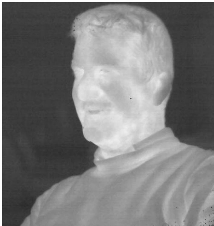
Figure 1.10: Image obtained by 384 \times 288 detector array fabricated at METU-MEMS Center with 35 \mu\text{m} pixel pitch.
