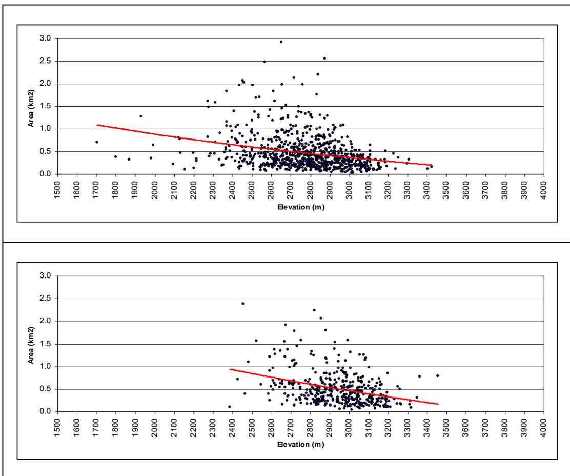
**Figure 5.10:** Scatter plots of elevation versus area of cirques for the northern (above) and southern (below) parts of the area.
