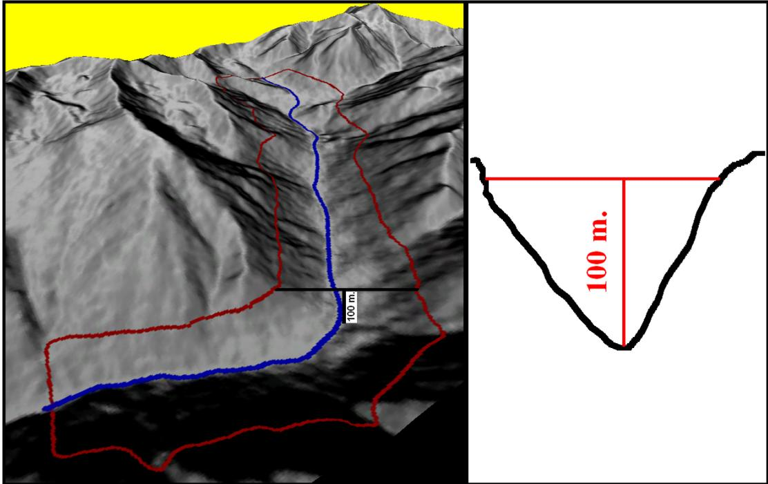
**Figure 4.4:** Determination of polygon by elevating the valley floor for 100 m.
