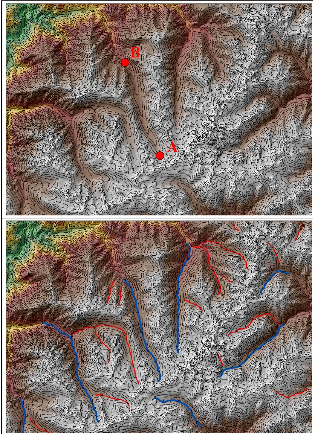
**Figure 4.1:** Determination of the glacial valleys over the DEM. The points A and B in the upper figure correspond to the starting and the ending points of the valley. The red and the blue lines are the glacial valleys (main and tributary) drawn for this example.
