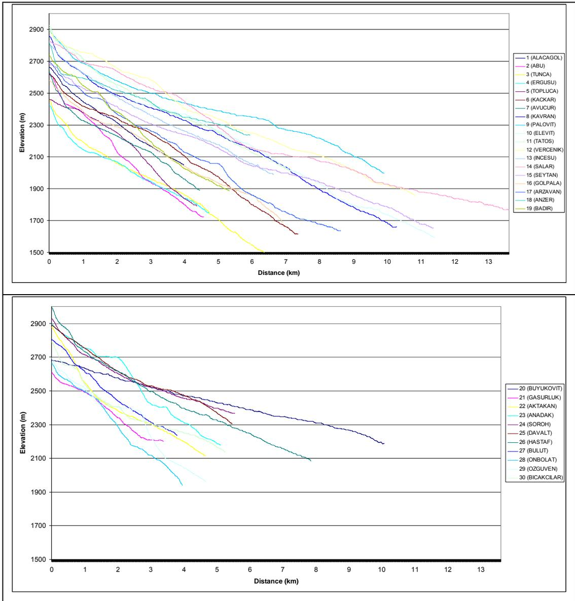
**Figure 4.12:** Longitudinal profiles of the valleys of the northern (upper) and the southern (lower) parts of the area.
