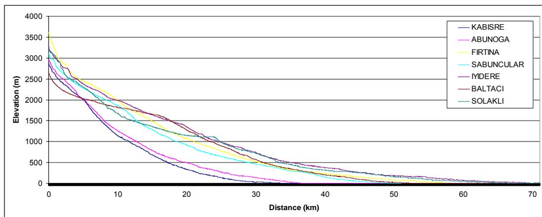
**Figure 3.4:** Overlapping longitudinal profiles of rivers on the northern side.
