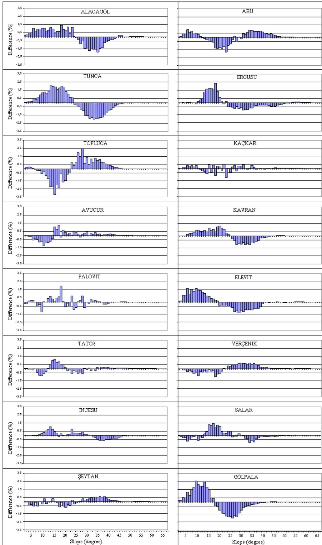
**Figure 4.14:** Histograms used to investigate the symmetry of glacial valleys by subtracting the western pixels from eastern ones.
