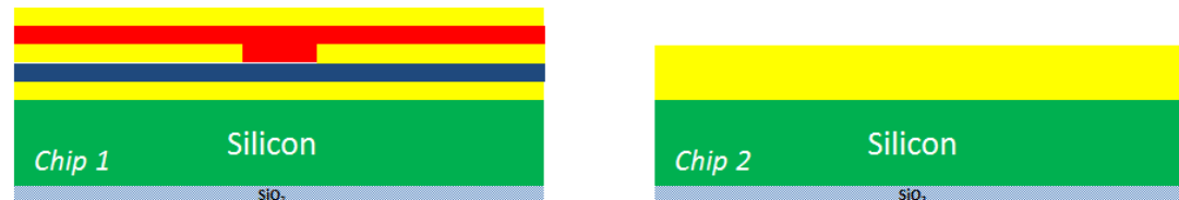
(e) Deposit 3 rd parylene layer
