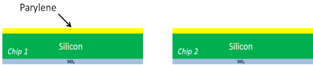
(a) Deposit 1 st parylene layer
