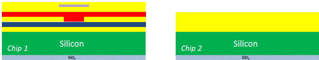
(g) Deposit and pattern final parylene layer
