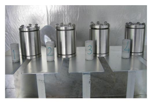
Fig D.3 Photograph of 4 cement plugs with four core holders
