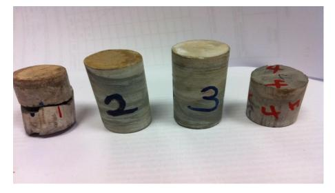
Fig H.1 Photograph of cement plugs after experiment
