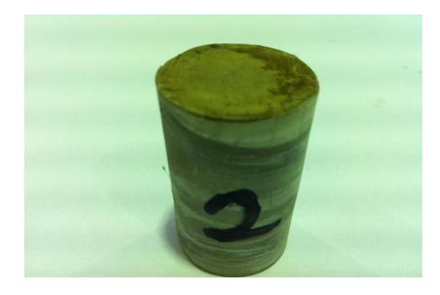
Fig H.3 Photograph of cement plug #2 after experiment
