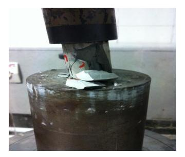
Fig 6.1 Cement plug 4 while applying vertical load
