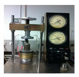
Fig G.1 Schematic of Versa-Tester Apparatus
