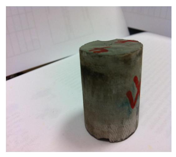
Fig H.5 Photograph of cement plug #4 after experiment
