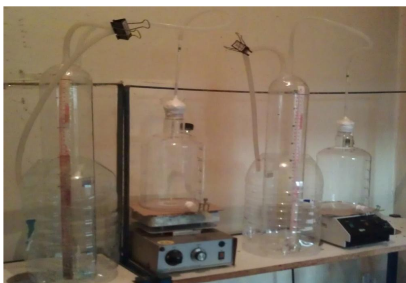
Figure 3-1: 2.5 liter anaerobic batch reactors
