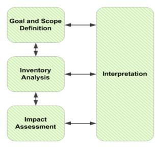
Figure 1. Phases of LCA [31]
