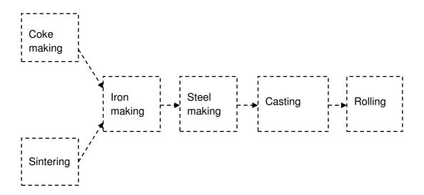
Figure 4. Flow diagram of integrated iron and steel production process
