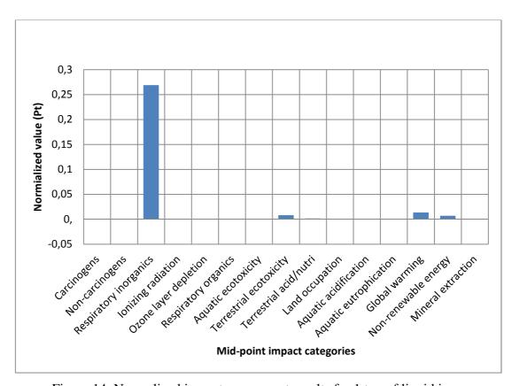
Figure 14. Normalized impact assessment results for 1 ton of liquid iron
