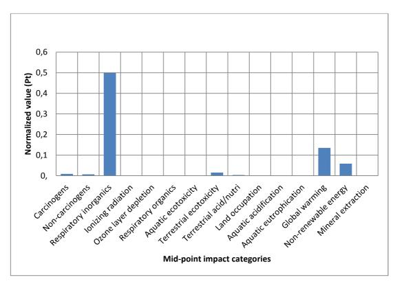
Figure 20. Normalized impact assessment results for 1 ton of wire rod
