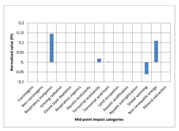
Figure 12. Normalized impact assessment results for 1 ton of coke
