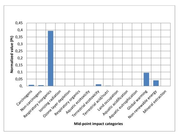
Figure 15. Normalized impact assessment results for 1 ton of liquid steel
