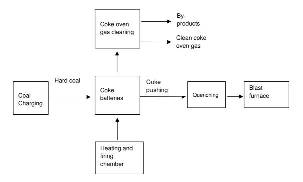
Figure 5. Flow diagram of Coke making
