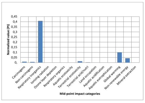
Figure 19. Normalized impact assessment results for 1 ton of slab
