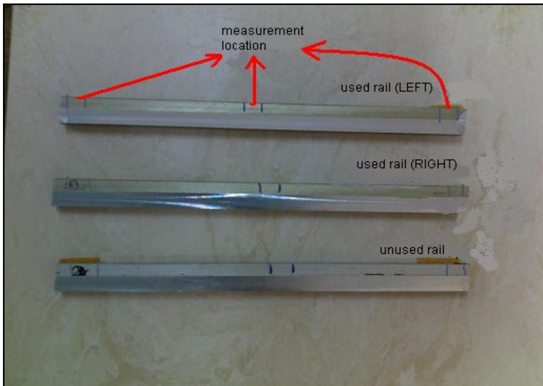
Figure 3-13 A view of measurement locations on the rails
