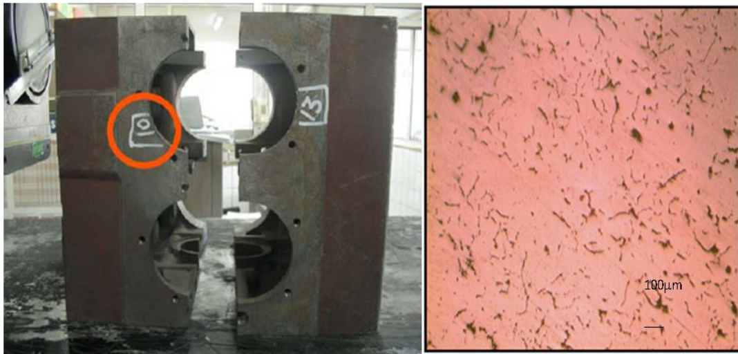
Figure 4.25 Section number 10 with 16.83 mm thickness had 22.89% nodularity. Nodularity value of section 10 may show differences in accordance with obtaining it near the runner or obtaining it far from the runner.
