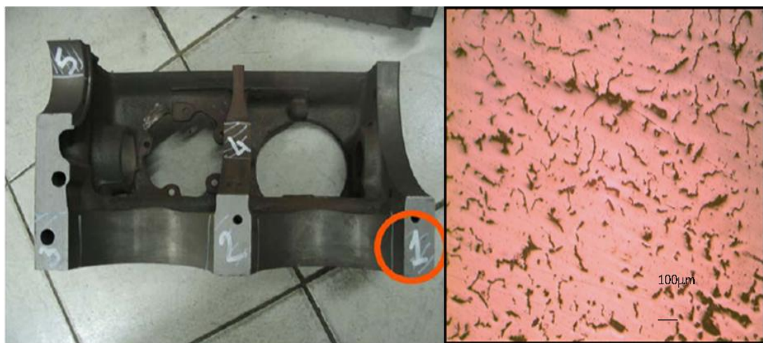
Figure 4.16 Section number 1 having 32.72 mm had 23.68% nodularity. Section 1 was placed near the runner. Moreover, it was one of the thickest sections of the diesel engine block.
