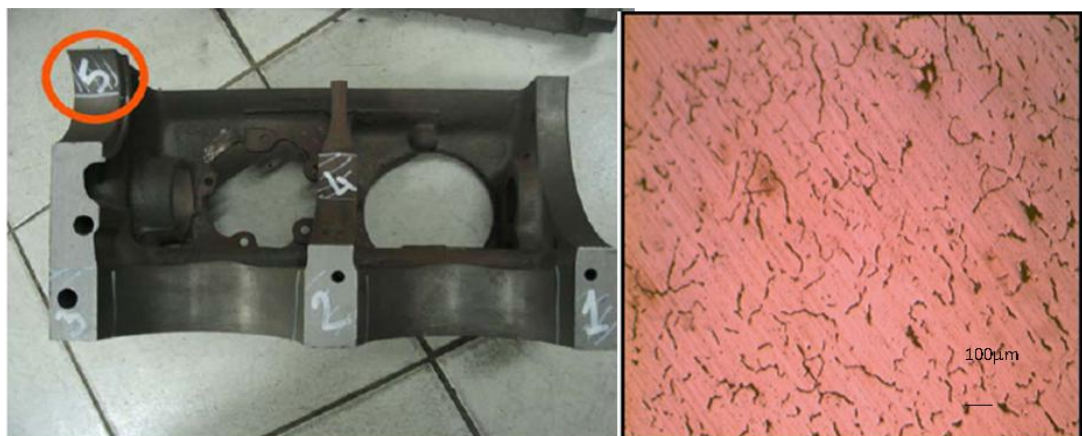
Figure 4.20 Section number 5 having 40.85 mm thickness had 30.13% nodularity. Though section 5 was the thickest section of the diesel engine block, it could include high nodularity% value due to its position in the mold cavity.
