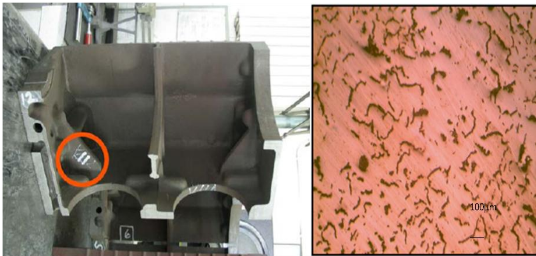
Figure 4.26 Section number 11 having 10.95 mm thickness had 20.39% nodularity. The things that have been told for section number 7 are suitable for section number 11.
