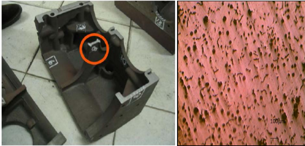
Figure 4.23 Section number 8 with 7.25 mm thickness had 26.33% nodularity. Section 8 generally consisted of higher nodularity percentage value than the other sections of the diesel engine block. This may seem normal due to its thickness.
