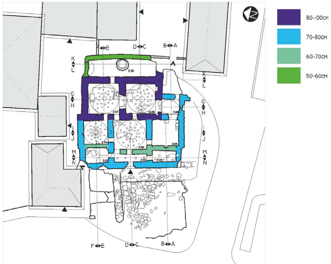
Figure 25, Load Bearing Wall Thickness Distribution
