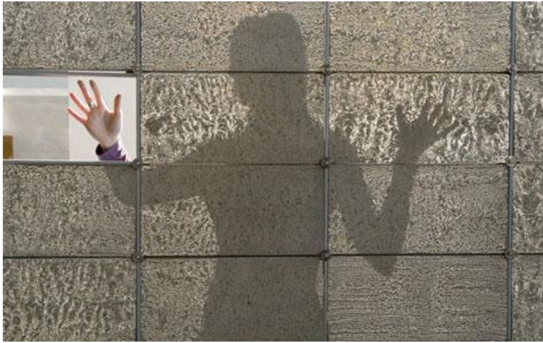
Figure 6. Light Transmitting Concrete by Aran Losonczi
