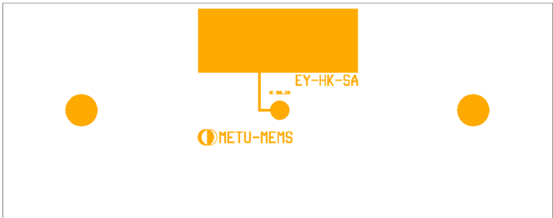
Figure A.8: Bottom electrode mask layout for normally closed electrostatic microvalves.
