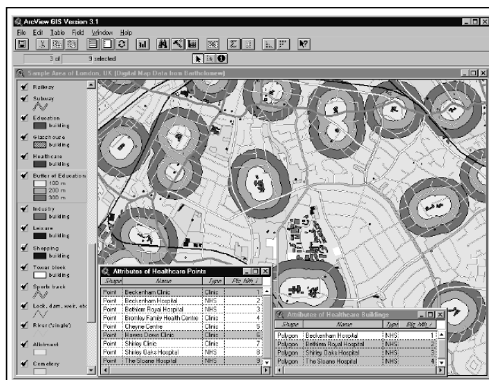
Figure 2.18. 100, 200 and 300 meters of constant deterministic Euclidian-based buffers around each educational facility in London, UK (Boulos et al. 2001)
