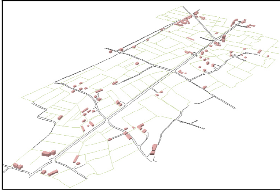
Figure 5.8. The result of the 3D digitizing process by using stereo image
