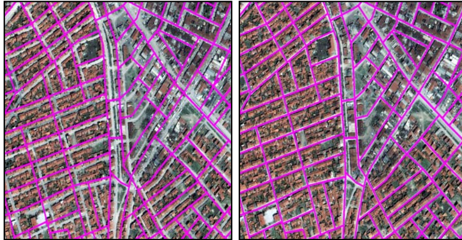
Figure 6.11. Rational function result at left hand side and satellite model result at right hand side
