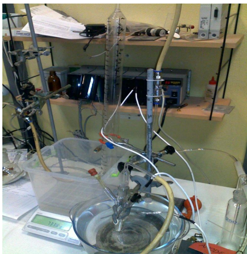
Figure 3-2 Picture of batch hydrogen generating system
