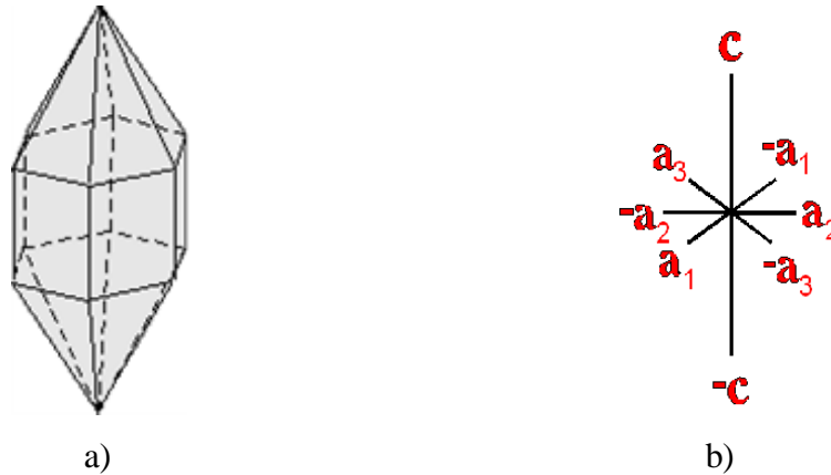
Figure 1.1. a) Hexagonal Dipyramidal shape [21]; b) Axial configuration of hexagonal shape [22].
