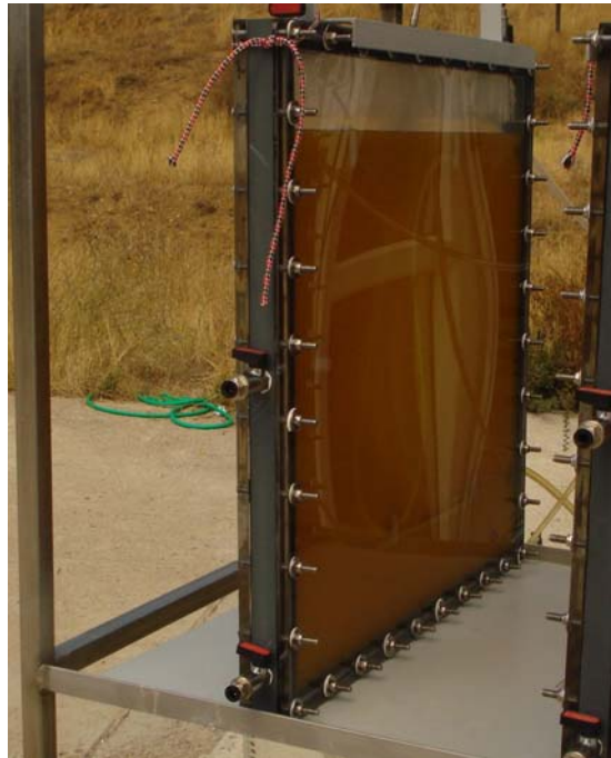
Figure 2.1 Picture of outdoor panel PBR (4L) with internal cooling coil run by Rb. capsulatus YO3 (hup - ) on DFESBTJ
