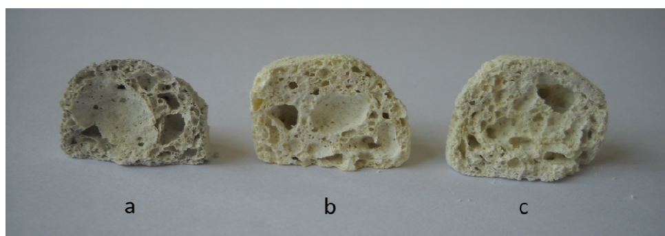
Figure 4.2 Pictures of a) plain, b) 10 wt % CaCO_3 added and c) 22.64 wt % colemanite added samples
