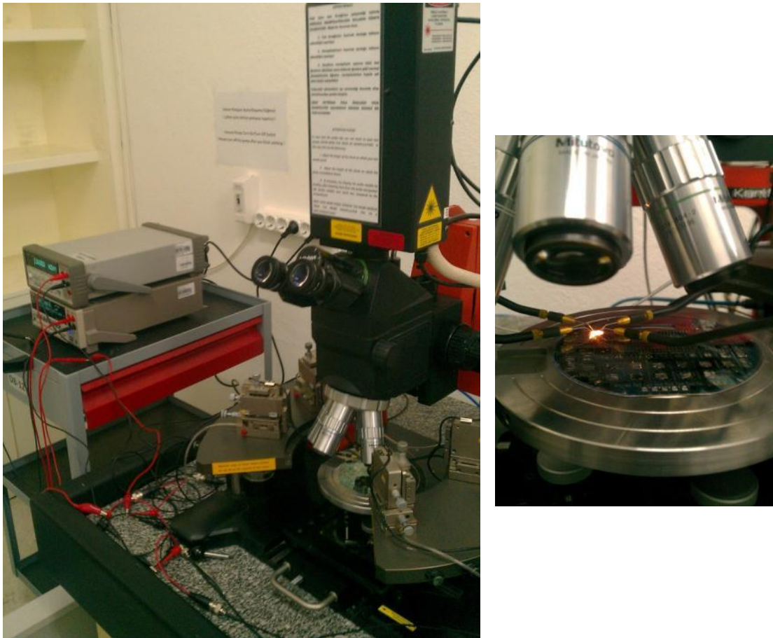
Figure 5.3. The test setup used for MEMS TE energy harvester performance measurement in steady state.
