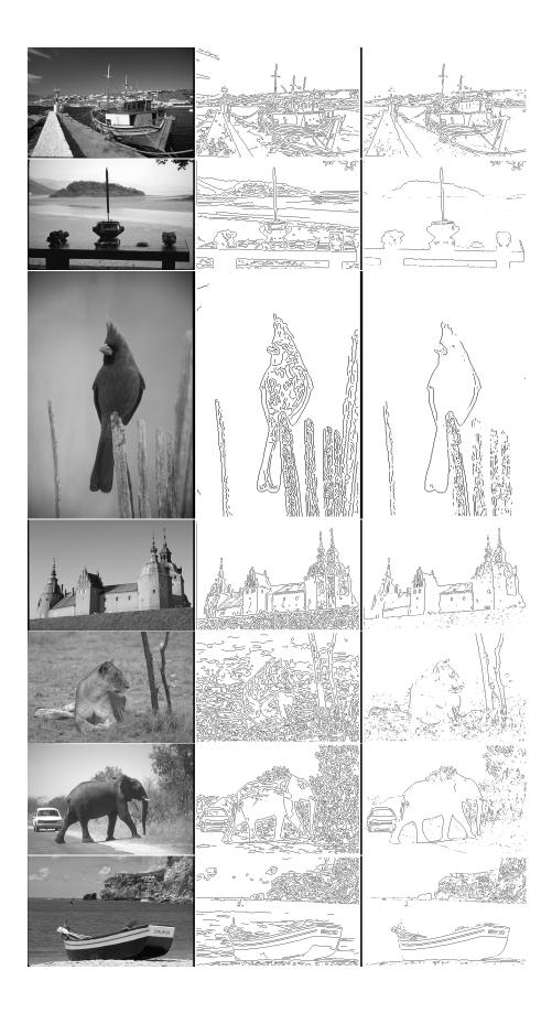
Figure 4.10: IC Results, images are ordered namely as original image, Canny, and IC on Canny.
