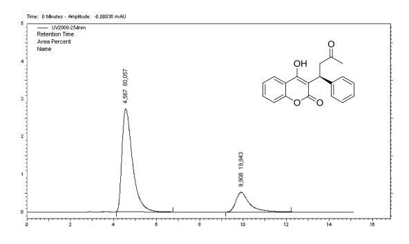
Figure A15. HPLC chromatogram of entry 3 in Table 3 (60% ee)
