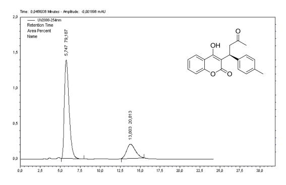
Figure A31. HPLC chromatogram of compound 10b (59.5% ee)
