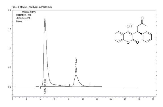
Figure A17. HPLC chromatogram of entry 4 in Table 5 (64% ee)
