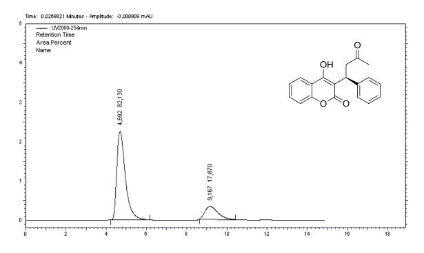
Figure A25. HPLC chromatogram of entry 6 in Table 9 (64.5% ee)
