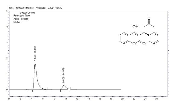
Figure A28. HPLC chromatogram of entry 1 in Table 11 (70% ee)
