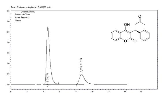
Figure A24. HPLC chromatogram of entry 4 in Table 9 (57.5% ee)
