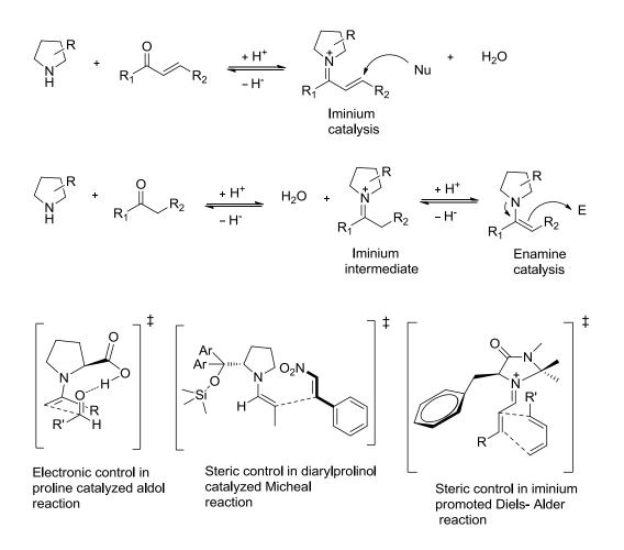
Scheme 9. Secondary amines in iminium and enamine catalysis
