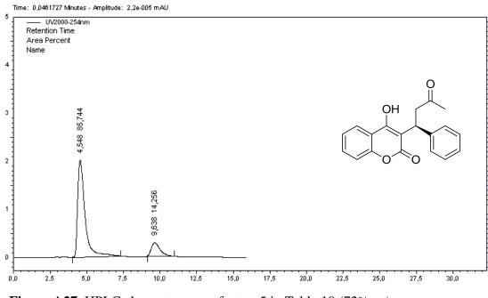
Figure A27. HPLC chromatogram of entry 5 in Table 10 (72% ee)
