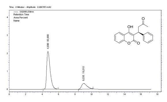
Figure A18. HPLC chromatogram of entry 8 in Table 6 (62% ee)
