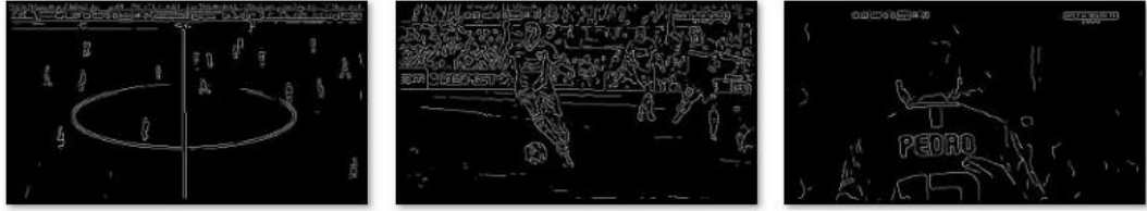
Figure 5 – Example images of edge pixels. Far view, Medium view, Close-up view [left-to-right].
