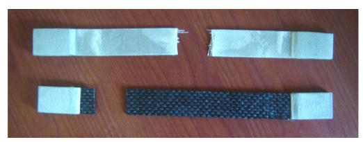
Figure C3: Specimens after the tensile tests
