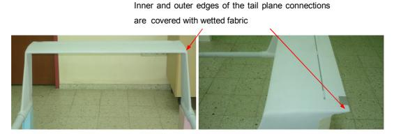
Figure 28: Permanent connection of the horizontal and vertical tail
