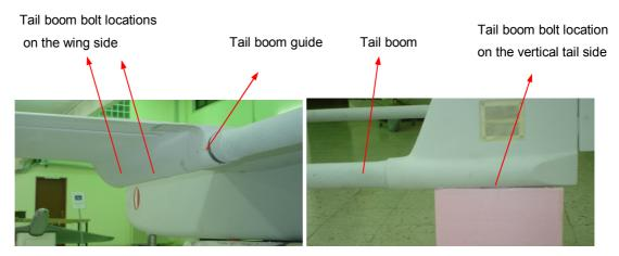
Figure 30: Tail boom bolt connection locations on the wing and the vertical tail
