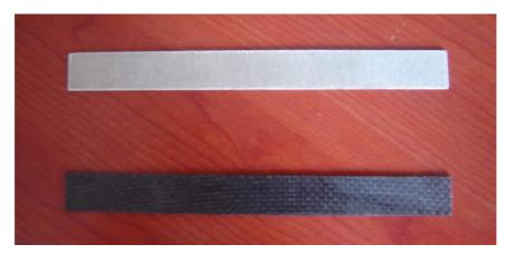
Figure C1: Specimens prepared according to ASTM D 3039/D 3039M
