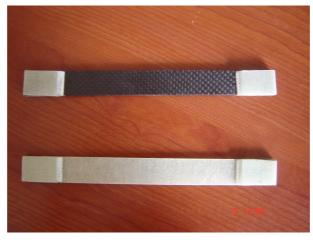
Figure C2: Specimens after tabs are glued
