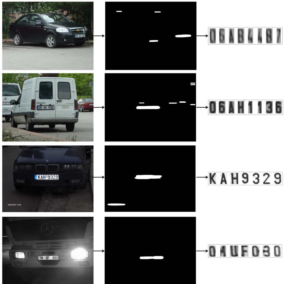
Figure 4.11: Successful license plate detection and character segmentation results for k = 2.5 , and K = 8 .
