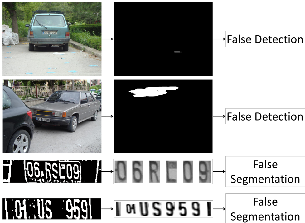
Figure 4.12: False license plate detection and character segmentation results for k = 2.5 , and K = 8 .
