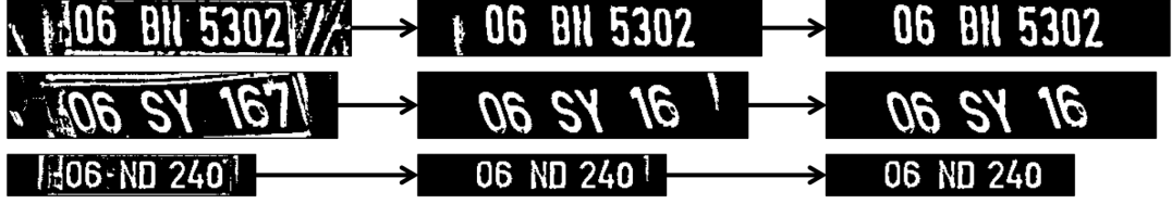
Figure 3.17: Results of inconsistent character placement elimination step. 1 st column: Segmentation output, 2 nd column: Individual blob analysis + character height consistency elimination output, and 3 rd column: Character placement consistency elimination results.
