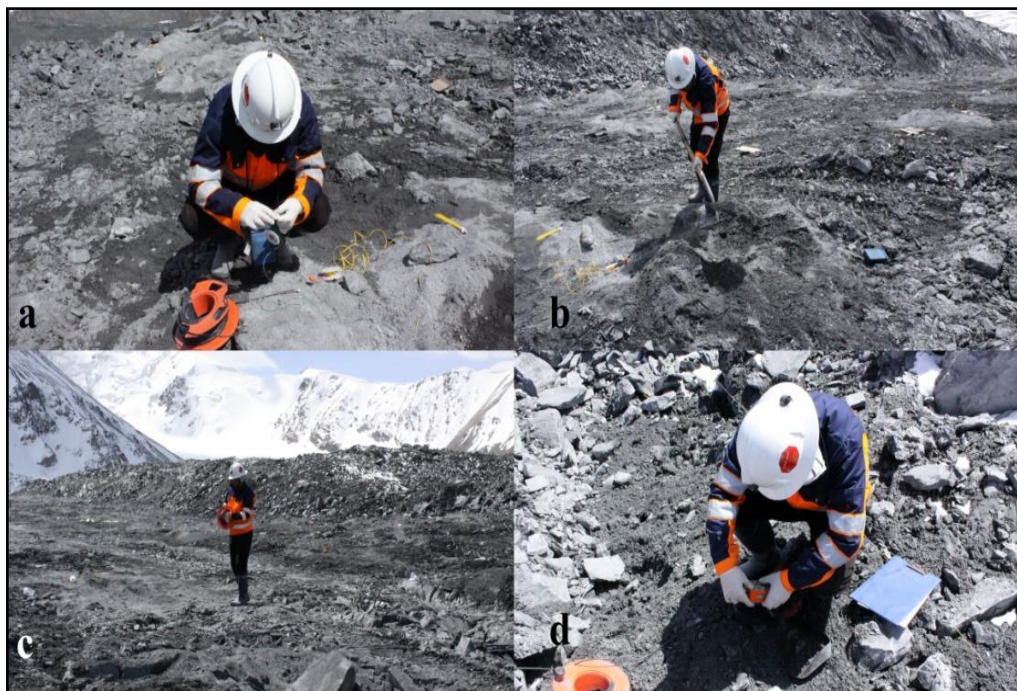
Figure 3.11 Setting equipments to measure in hole VOD
