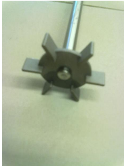
Figure 5.1.3 Rushton Turbine and the Impeller
