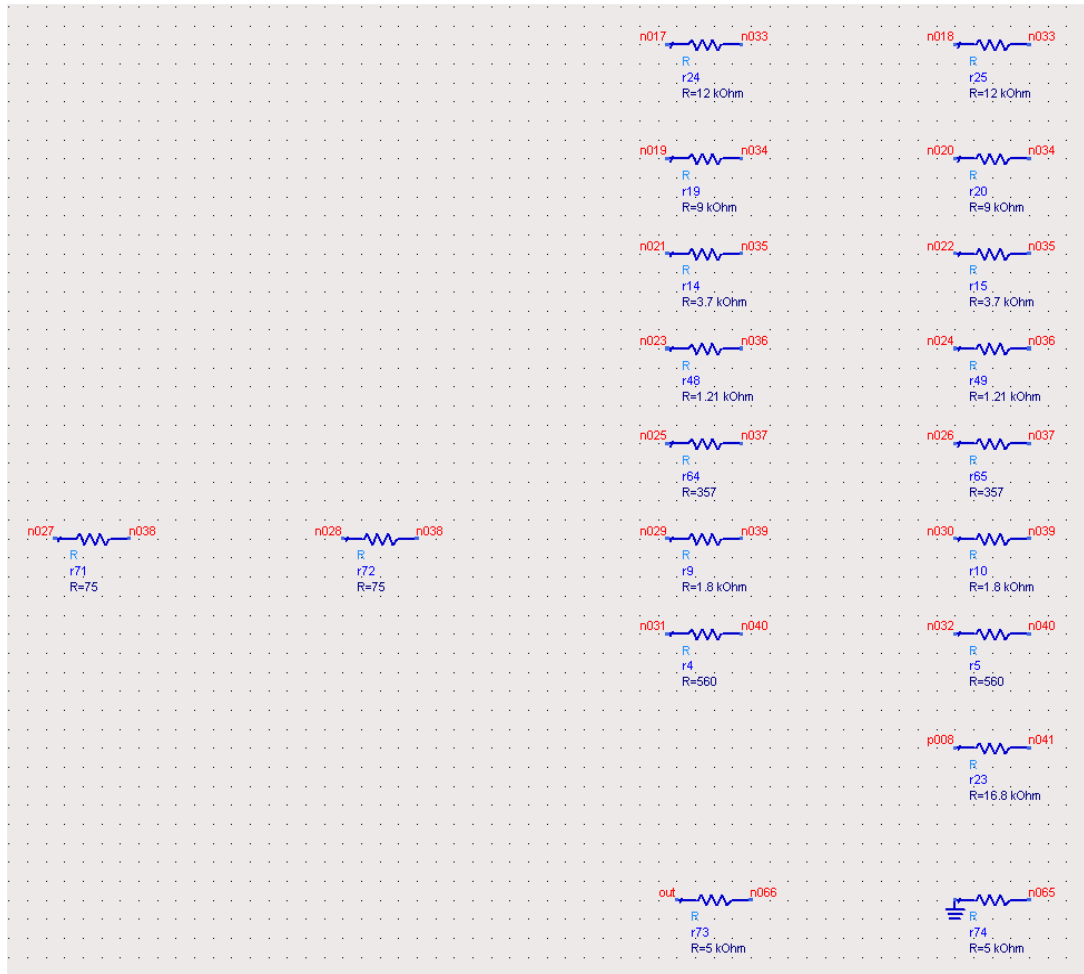
Figure 4-15: Modified resistor values for a better logarithmic response with smaller logarithmic error
