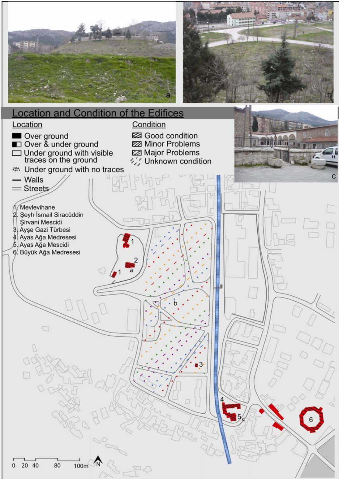
Figure 40: Location and Condition of the Edifices in Area 1. a), b) and c) author, march 2011
