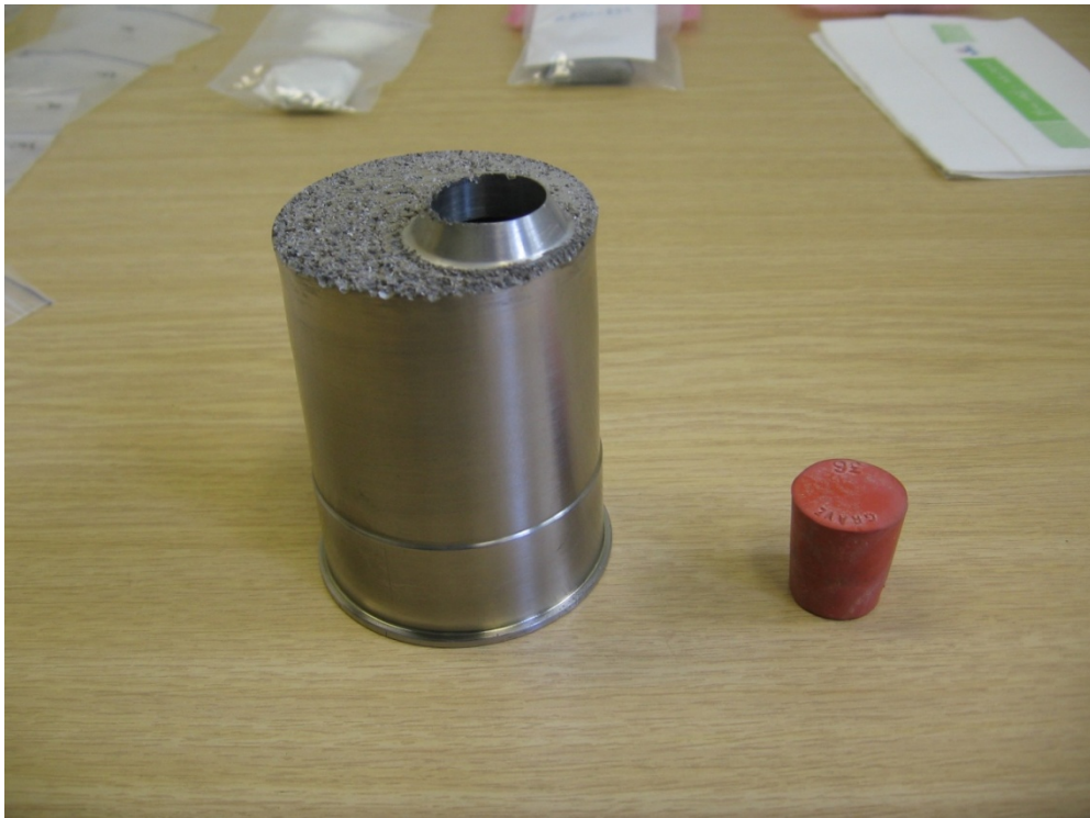
Figure 4.5 Calibration reservoir for adjustment of the rain fall rate.
