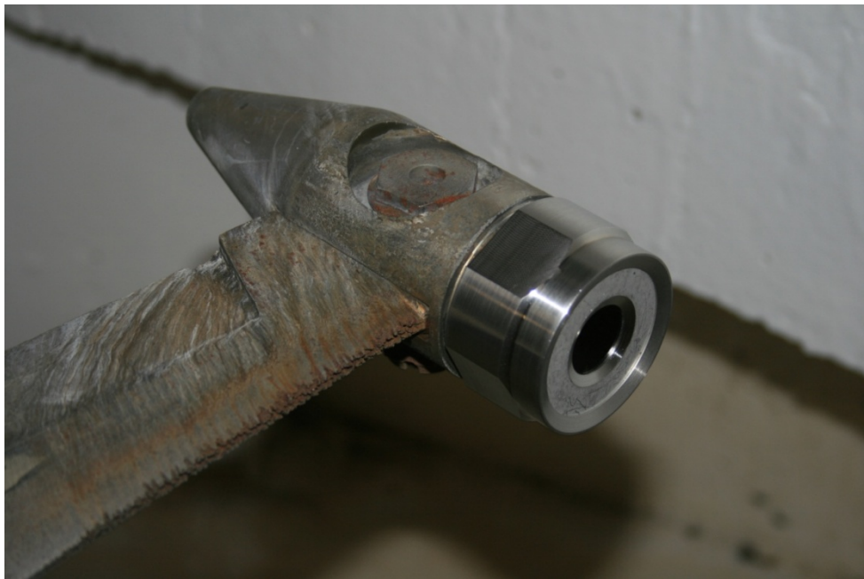
Figure 4.4 Mounting of the test specimen on end of the rotating arm.
