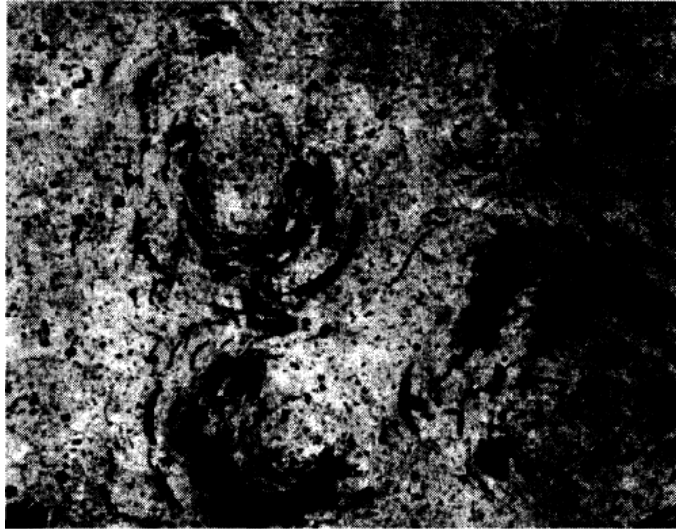
Figure 1.4 Rain erosion damage.
