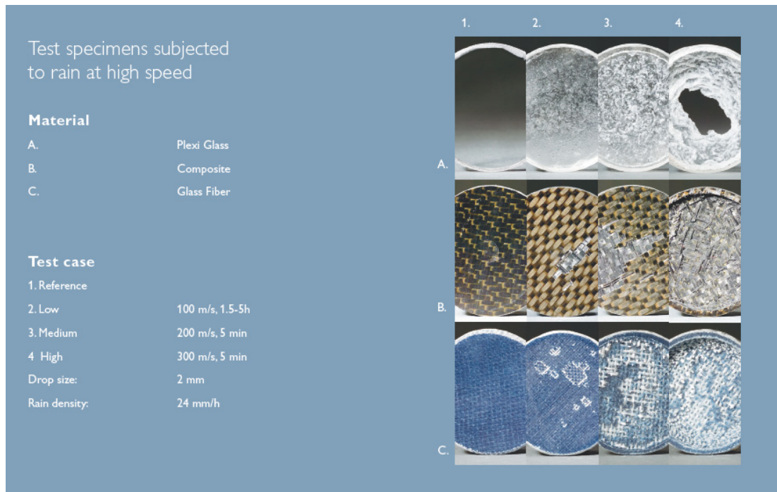
Figure 4.6 Test specimens subjected to rain at high speed [43].
