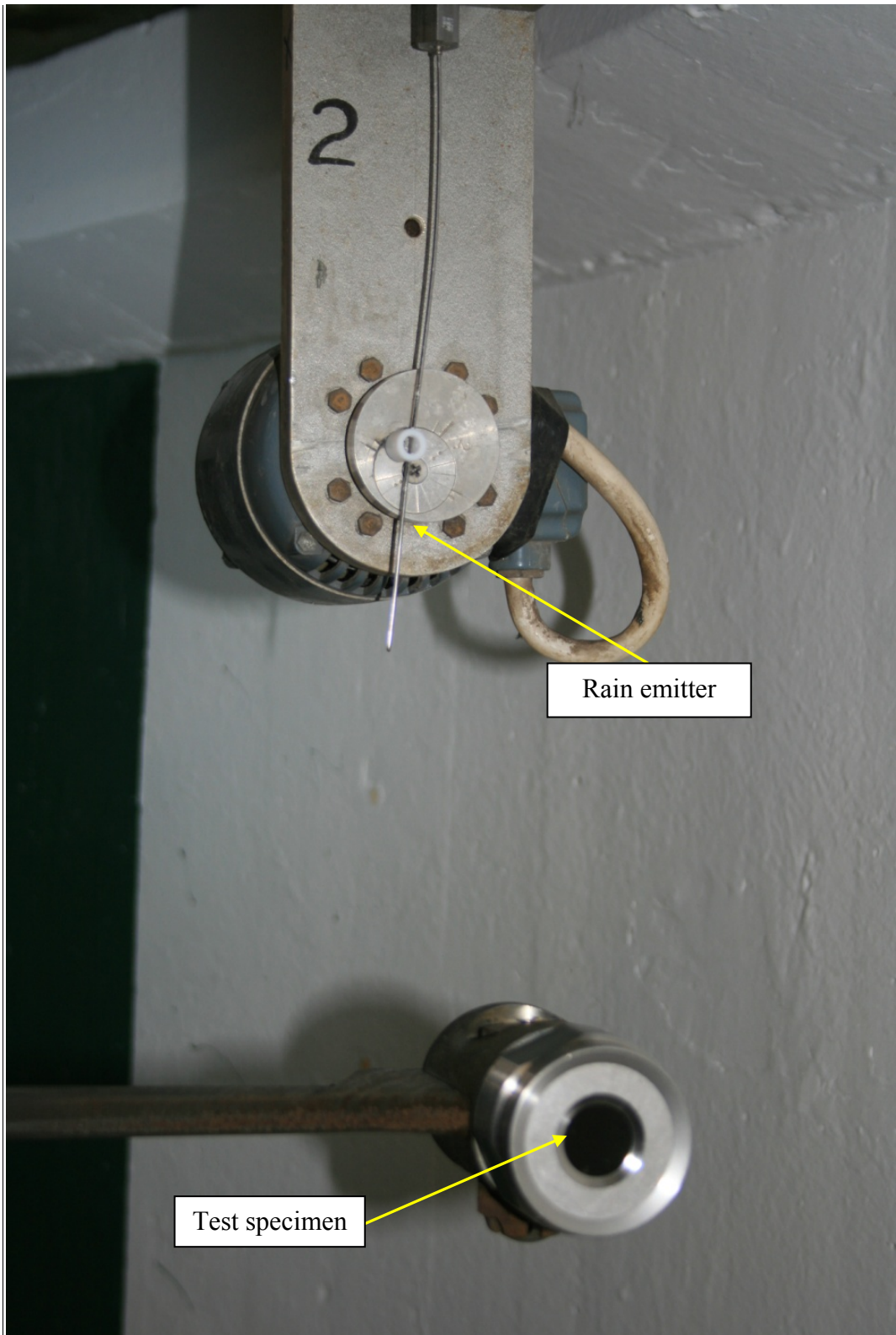
Figure 4.3 When the test specimen passes below a rain emitter.
