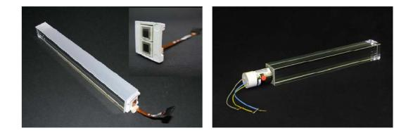
Figure 3.8: Lead tungstate crystals with photodetectors attached. Left: A crystal in barrel inserted a capsule with two APDs. Right: A crystal in endcap with a VPT attached.
