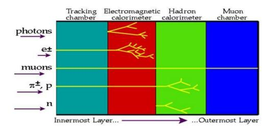
Figure 3.4: The CMS detector layers.
