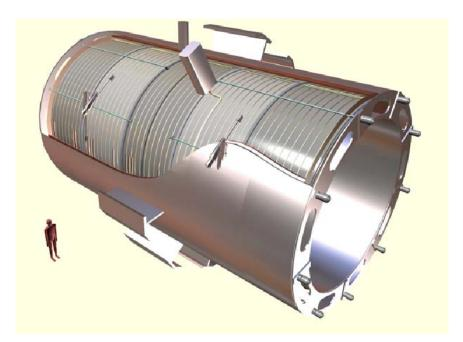
Figure 3.11: Superconducting magnet of CMS.
