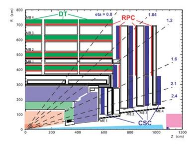
Figure 3.10: Longitudinal view of the muon system.
