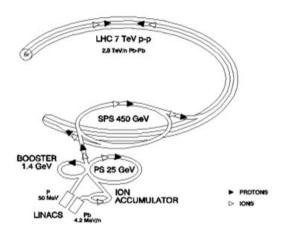
Figure 3.2: CERN Accelerator Complex.
