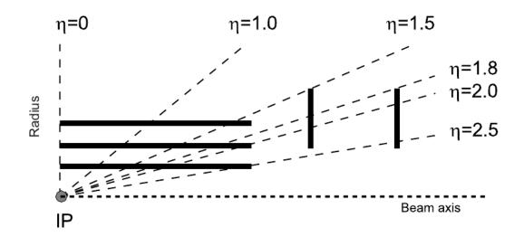
Figure 3.5: Geometrical layout of the pixel detector.
