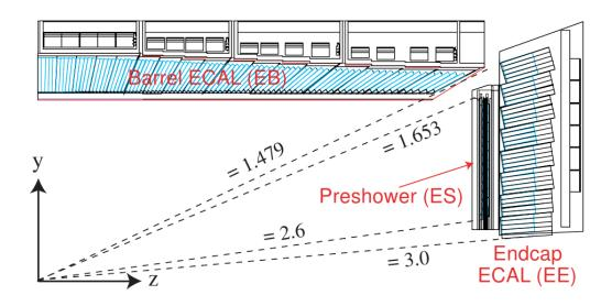
Figure 3.7: Transverse view of the electromagnetic calorimeter (ECAL).
