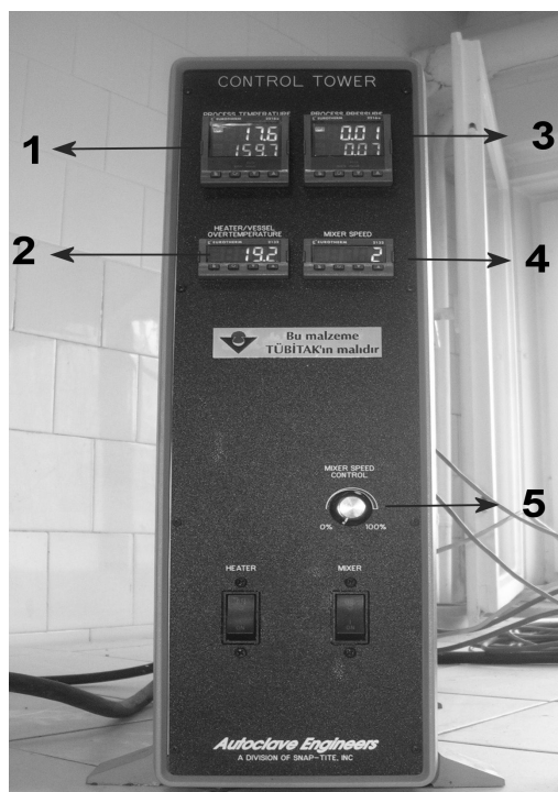
Figure 2.2 Control unit (Cizmeci, 2007)
