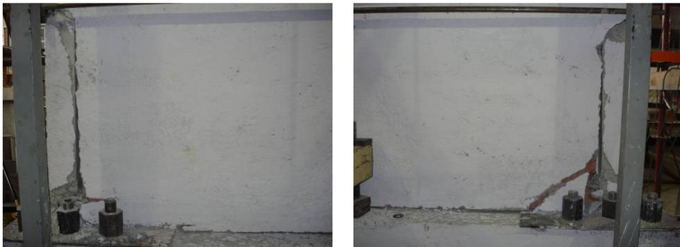
**Figure 5.91.** Rear Side Views at the End of Eighteenth Load Reversal, Specimen **WSP**
