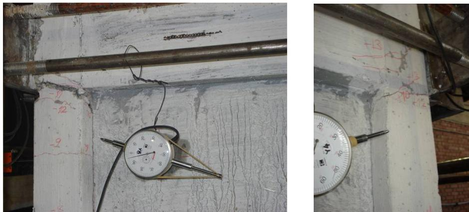
**Figure 5.90.** Views of First Storey Beam-Column Joints at the End of Thirteenth Load Reversal, Specimen **WSP**
