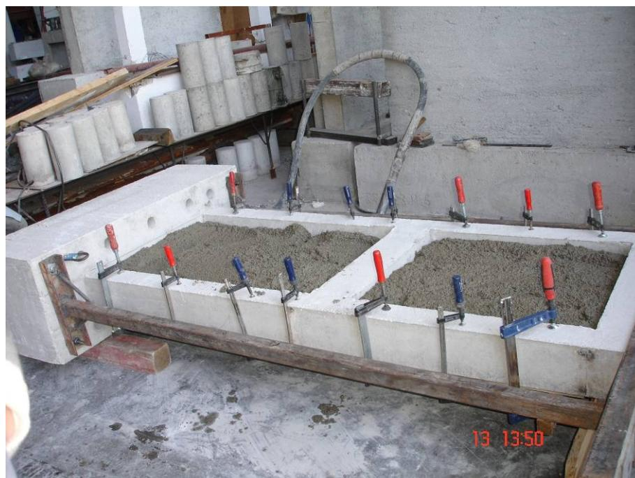
**Figure 3.2.** Cast-in-place RC Infill Preparation for Specimen NRC
