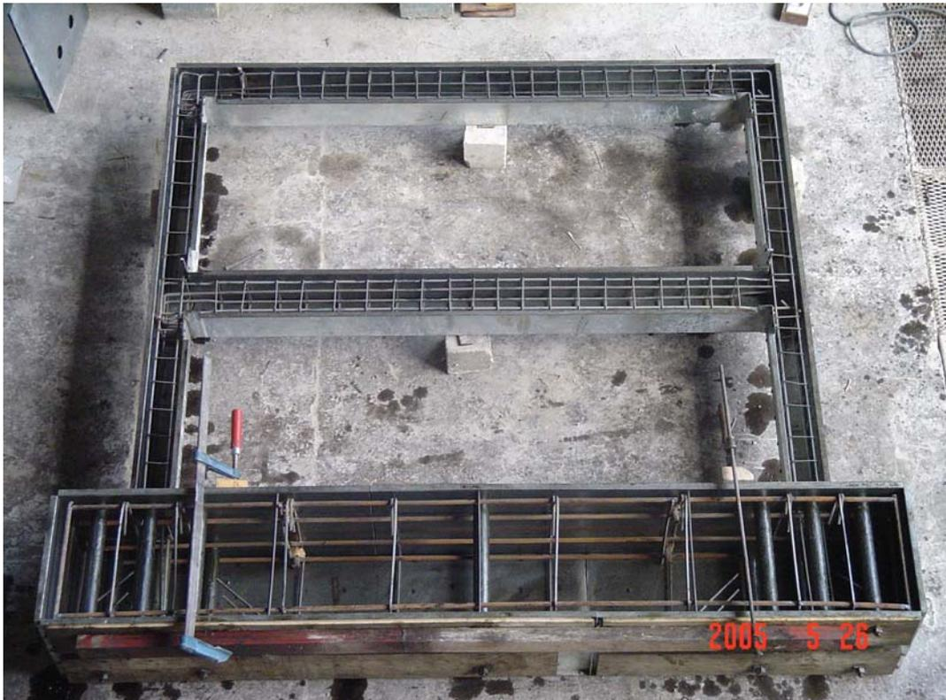
**Figure 3.17.** Reinforcement Details of Wider Series Specimens (dimensions in mm)
