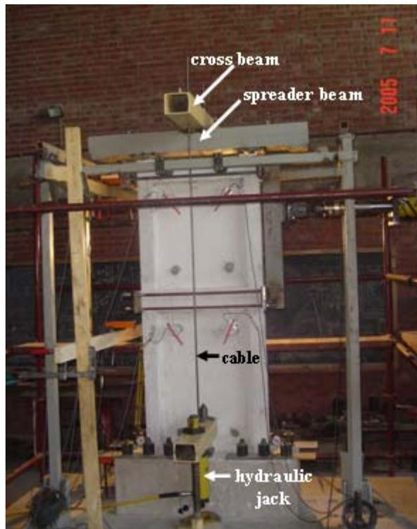
**Figure 4.6.** Vertical Loading System
