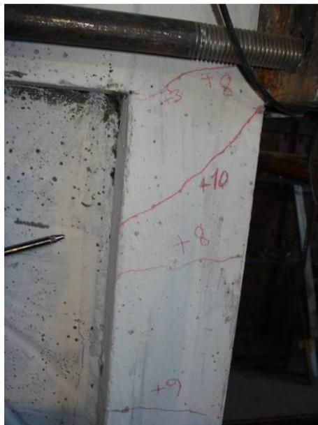
**Figure 5.98.** Diagonal Shear Crack on First Storey North Column at the End of Tenth Load Reversal, Specimen **WRC**
