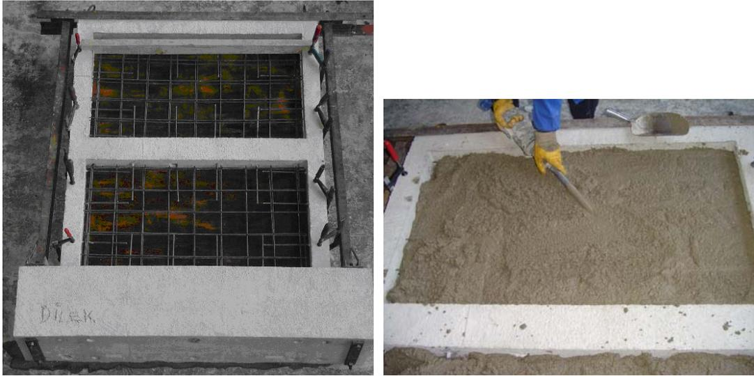
**Figure 3.40.** Views from Production Stages of Specimen SRC
