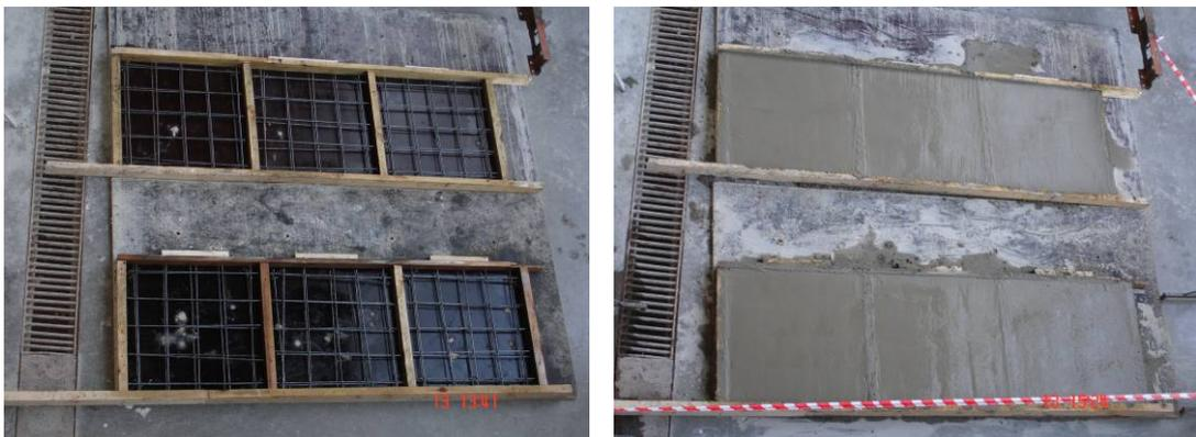
**Figure D.5.** Views from **RC** Infill Panel Specimen Preparations
