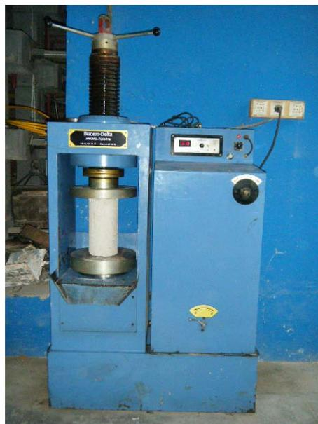
**Figure 3.3.** Compressive Strength Test of Cylinder Concrete Specimens
