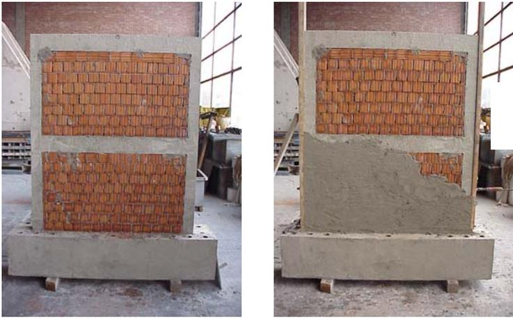
**Figure 3.27.** Hollow Clay Brick Infill Wall Workmanship (Ducarci, 2003)
