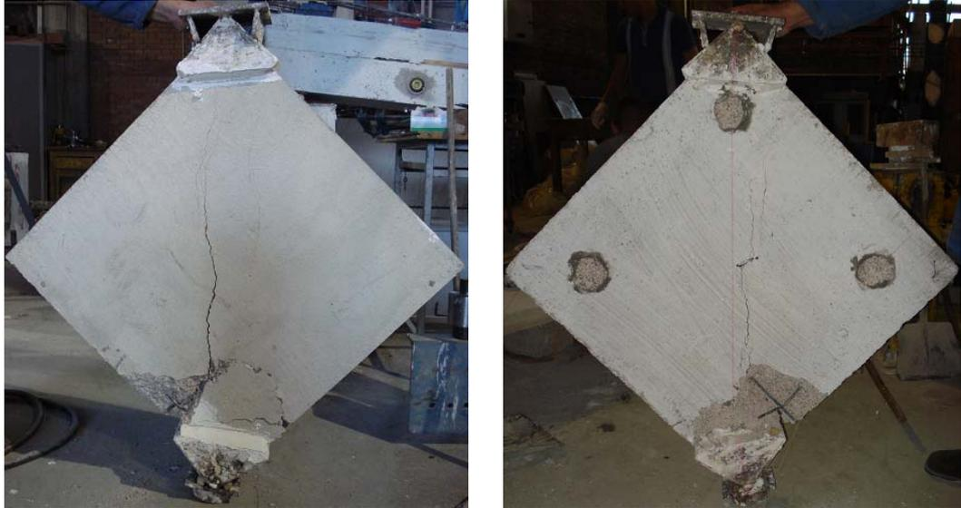
**Figure D.30.** Front and Rear Side Views of Specimen **RC2** after the Experiment
