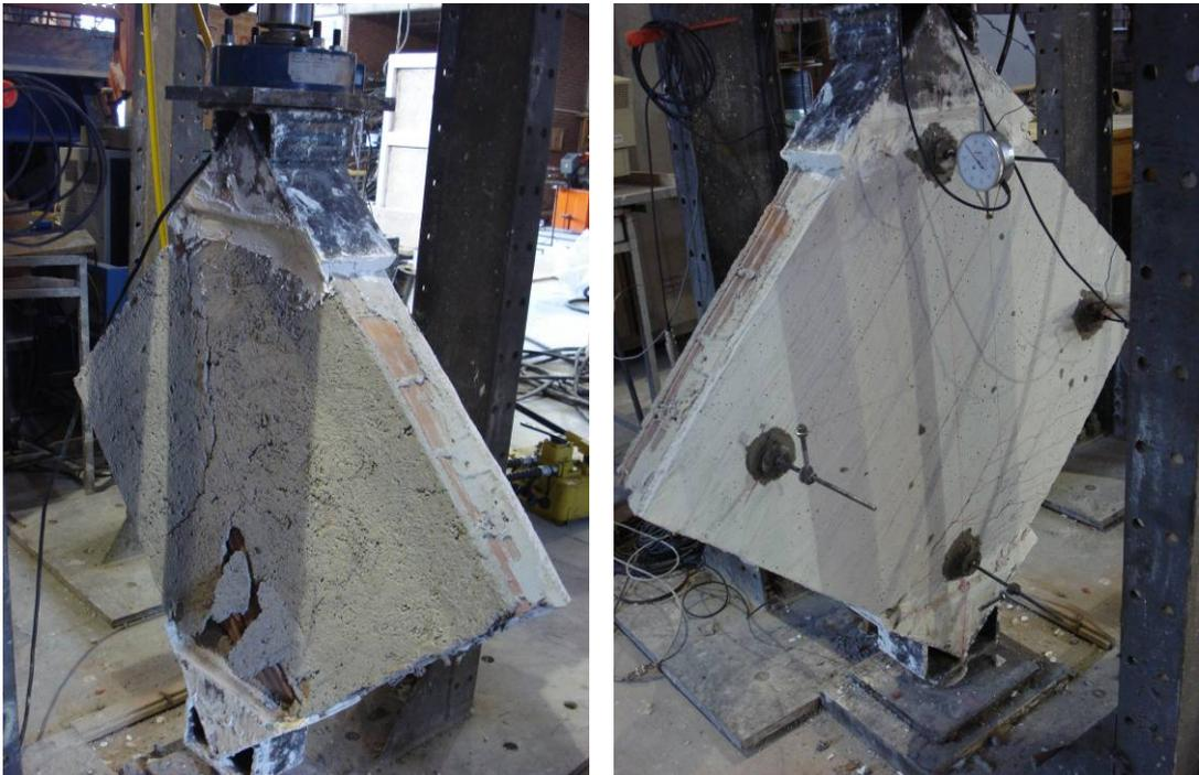
**Figure D.25.** Front and Rear Side Views of Specimen **SPS1** after Test
