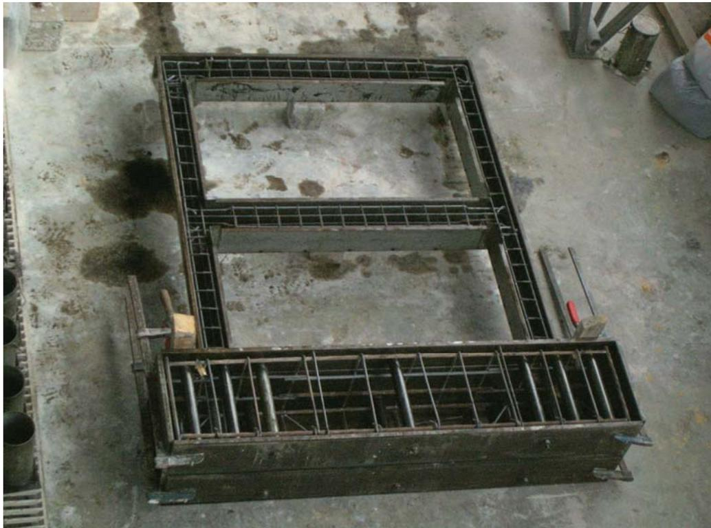
**Figure 3.15.** Reinforcement Details of Standard Series Specimens (dimensions in mm)
