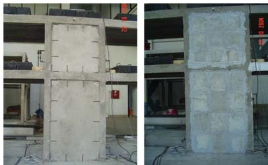
**Figure 5.104.** General Views from PC Panel Application to 3D Specimen
