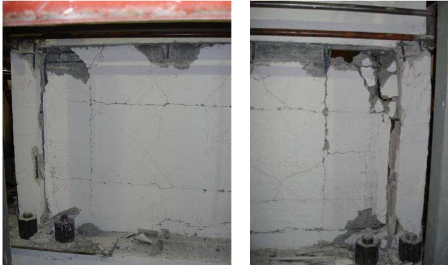
**Figure 5.100.** Views of First Storey Beam-Column Joints at the End of Eighteenth Load Reversal, Specimen **WRC**
