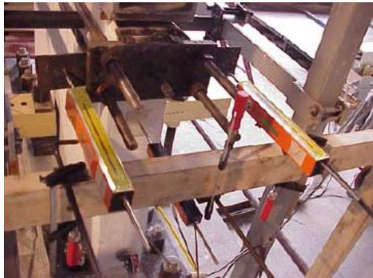
**Figure 4.17. LVDT's Fixed to the Timber Frame (Süsoy, 2004)**
