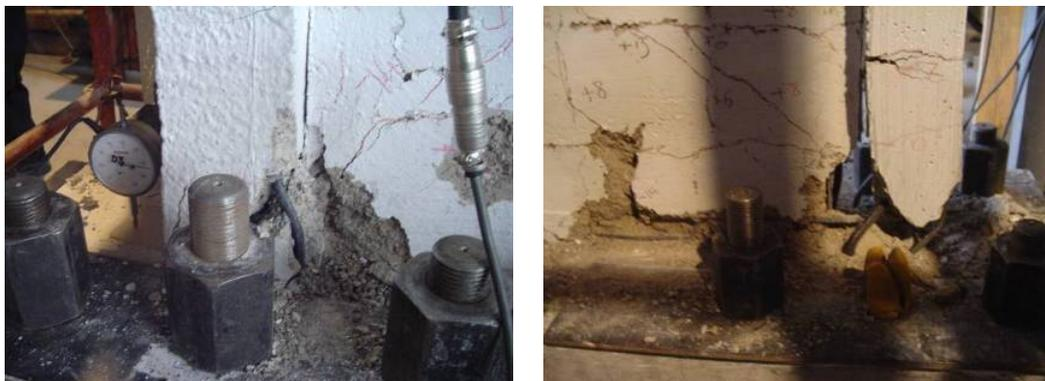
**Figure 5.64.** Buckling of the Longitudinal Reinforcement on Both North and South Column Bases at the End of Seventeenth Load Reversal, Specimen SRC
