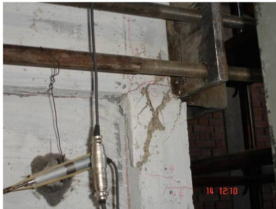
**Figure 5.83.** View of First Storey Beam-North Column Joint at the End of Fourteenth Cycle, Specimen **WRP**
