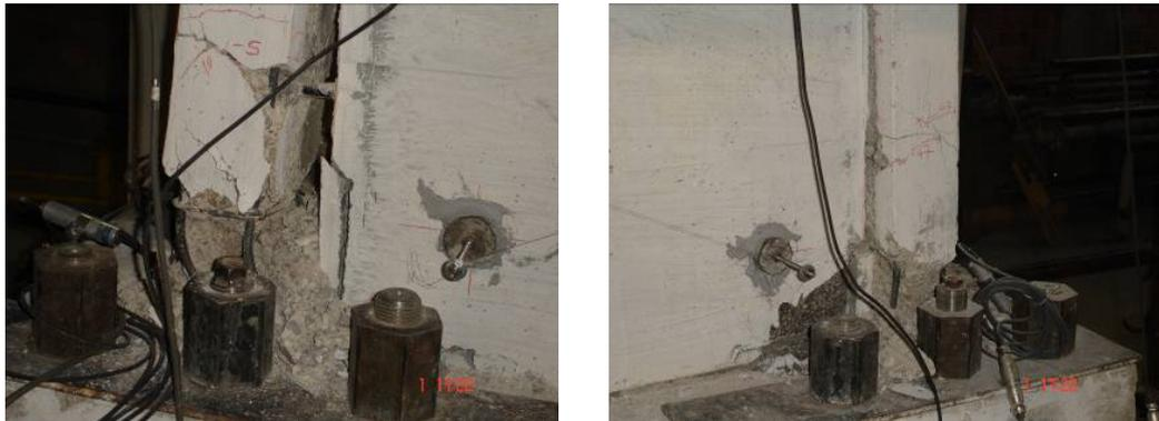
**Figure 5.48.** Views of Both Column Bases at the End of Sixteenth Load Reversal, Specimen **SRP**
