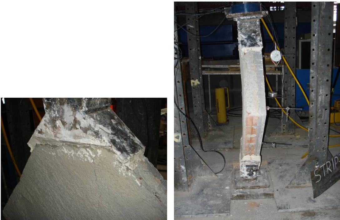
**Figure D.27.** Front and Rear Side Views of Specimen **SPS3** after Test
