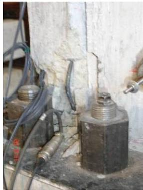
**Figure 5.57.** Buckling of the Longitudinal Column Reinforcement on the South Column Base at the End of Eighteenth Cycle, Specimen **SSP**
