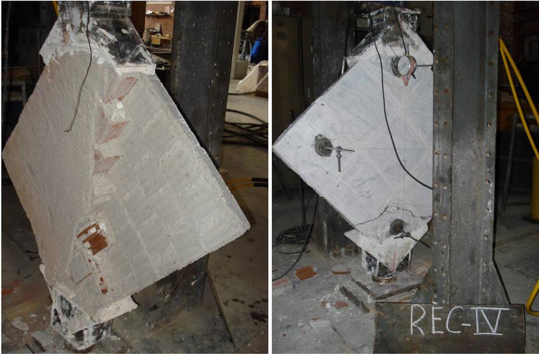
**Figure D.24.** Front and Rear Side Views of Specimen **RSP4** after Test
