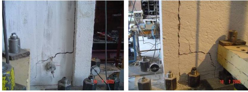
**Figure 5.24.** Panel and Plaster Cracks after Fifth Forward half cycle, Specimen NSP
