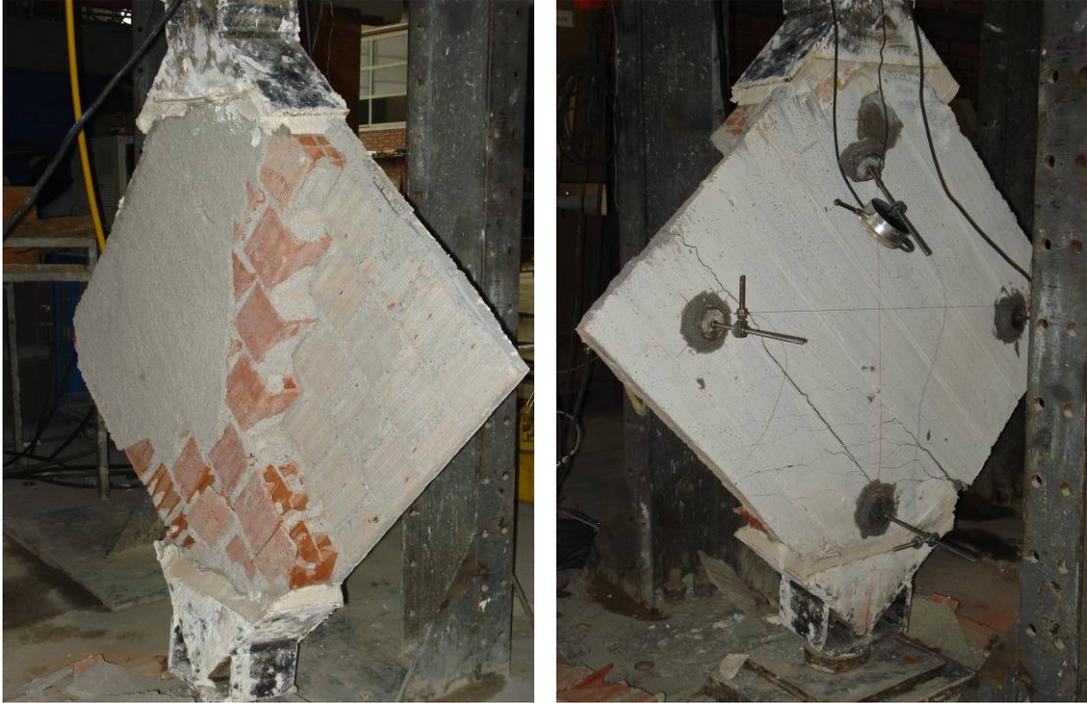
**Figure D.26.** Front and Rear Side Views of Specimen **SPS2** after Test
