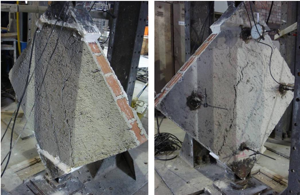
**Figure D.19.** Front and Rear Side Views of Specimen **HBP2** after Test
