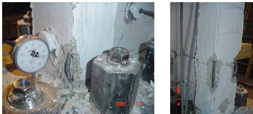
**Figure 5.17.** Buckling of Longitudinal Reinforcement at South and North Column Bases, Specimen NRP
