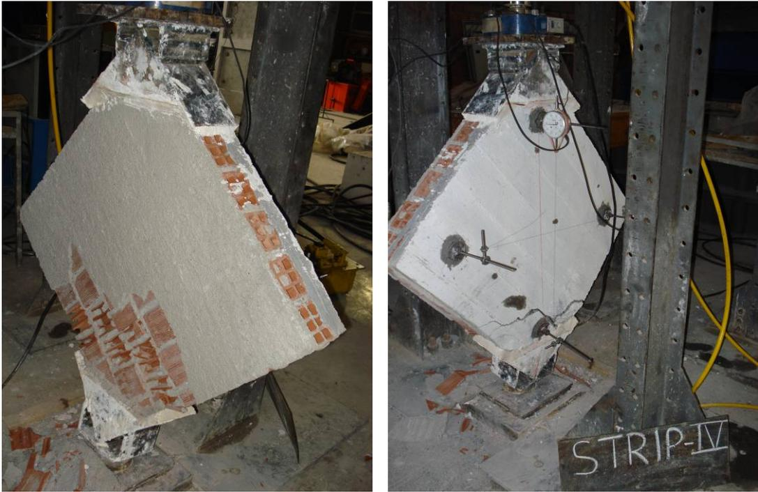
**Figure D.28.** Front and Rear Side Views of Specimen SPS4 after Test
