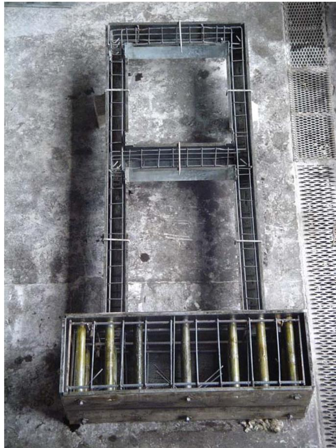
**Figure 3.13.** Reinforcement Details of Narrower Series Specimens (dimensions in mm)
