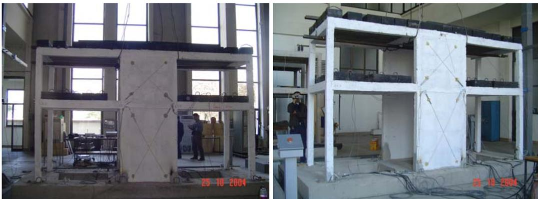
**Figure 5.110.** Front and Rear Side views of PC panel strengthened specimen SS at the end of Dynamic Testing Series
