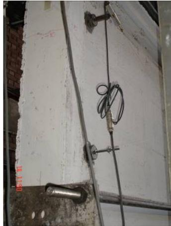
**Figure 5.82.** Crack on Second Storey South Column at the End of Tenth Cycle, Specimen **WRP**
