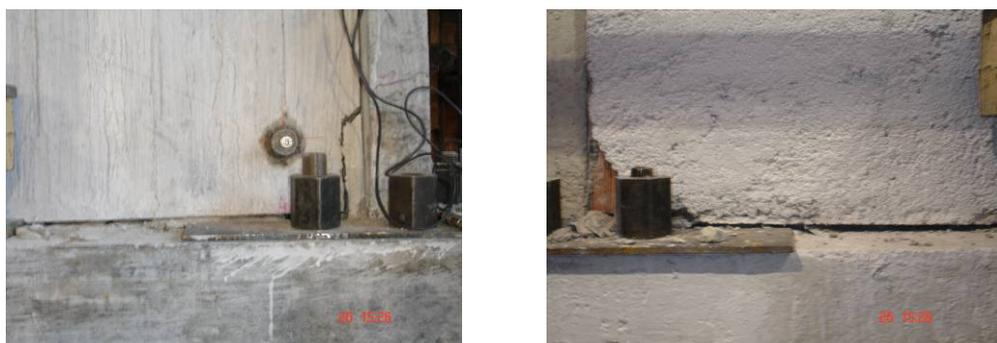
**Figure 5.56.** Front and Rear Side Views of Infill Panel Separation after Sixteenth Cycle, Specimen SSP
