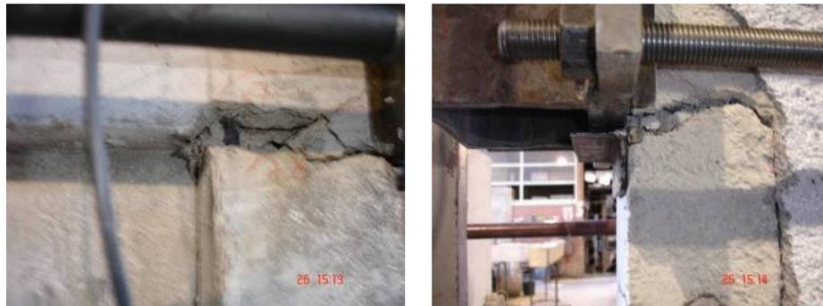
**Figure 5.55.** Front and Rear Side Views of First Storey Beam-North Column Joint at the End of Fifteenth Cycle, Specimen SSP
