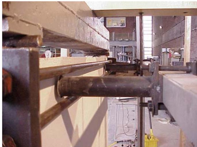
**Figure 4.5.** Ball Transfer Units
