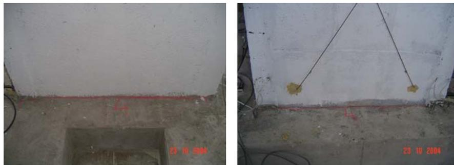
**Figure 5.107.** Separations of the Mid-bay Base due to Rocking
