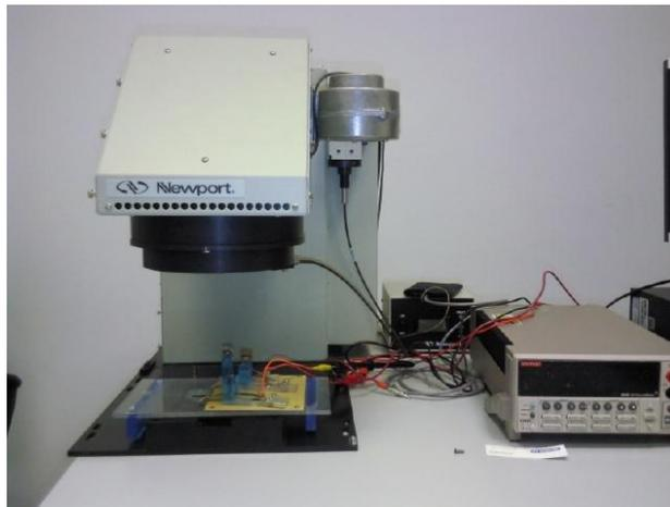
Figure 3.2-7: Solar simulator used for JV analysis of the cells deposited by sputtering.
