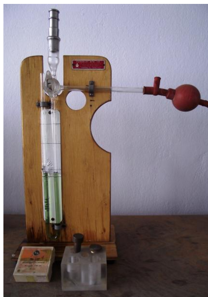
Figure 5. 3 Blaine air permeability apparatus to determine specific surface area of powder material (METUMEL)
