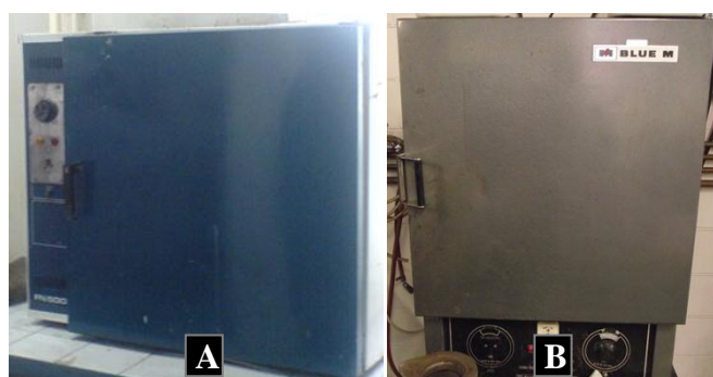
Figure 5. 20 Laboratory ovens used to dry pellets A) direct heating chamber used in METUMEL B) indirect heating chamber used in MTUCEL
