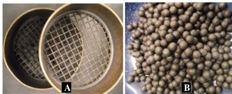
Figure 5. 19 A) 12.7 mm (0.500 inch) and 11.2 mm (0.441 inch) standard sieves to control the pellet size and B) wet pellets produced in MTUCEL
