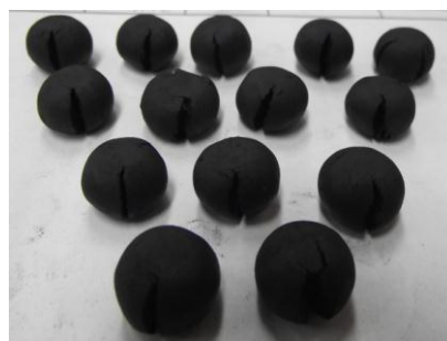
Figure 6. 25 Wet pellets with high degree of plasticity after drop number test and wet compressive strength measurement
