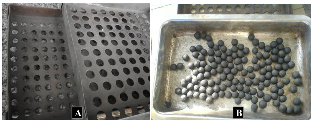
Figure 5. 18 A) 12.0 mm and 10.0 mm special screens to control the pellet size and B) wet pellets produced in METUMEL
