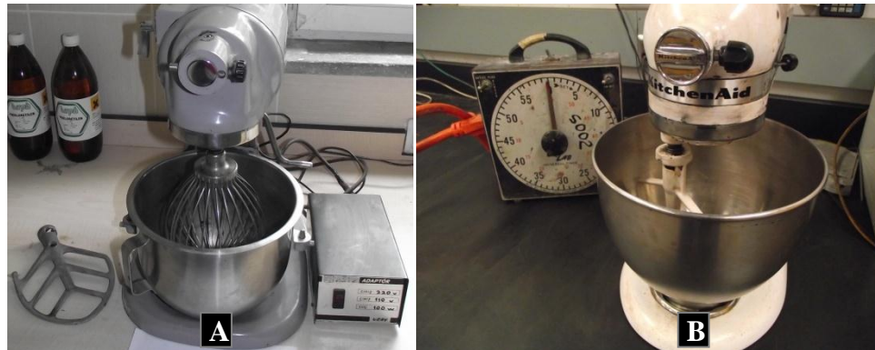
Figure 5. 16 A) Mixer used in METUMEL B) kneader-mixer used in MTUCEL to mix raw materials
