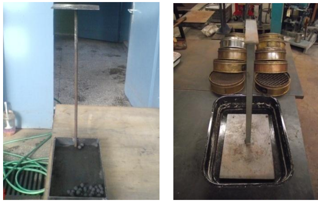
Figure 5. 21 Steel plates used to determine drop number from 46 cm of wet pellets
