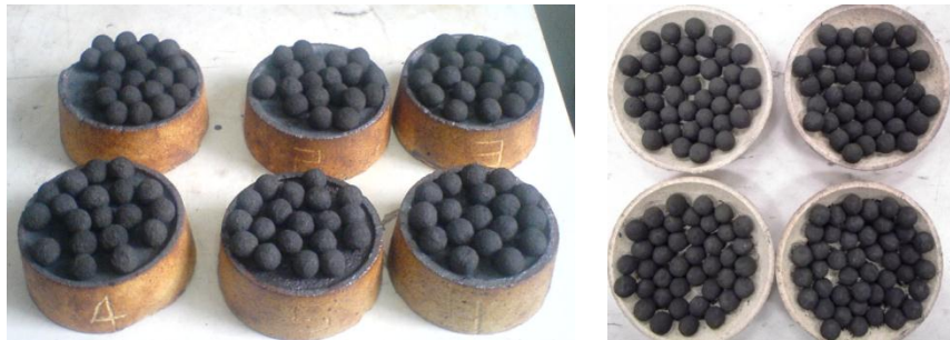
Figure 5. 25 Dry pellets, in one layer, in plate type crucibles before preheating or firing in furnace
