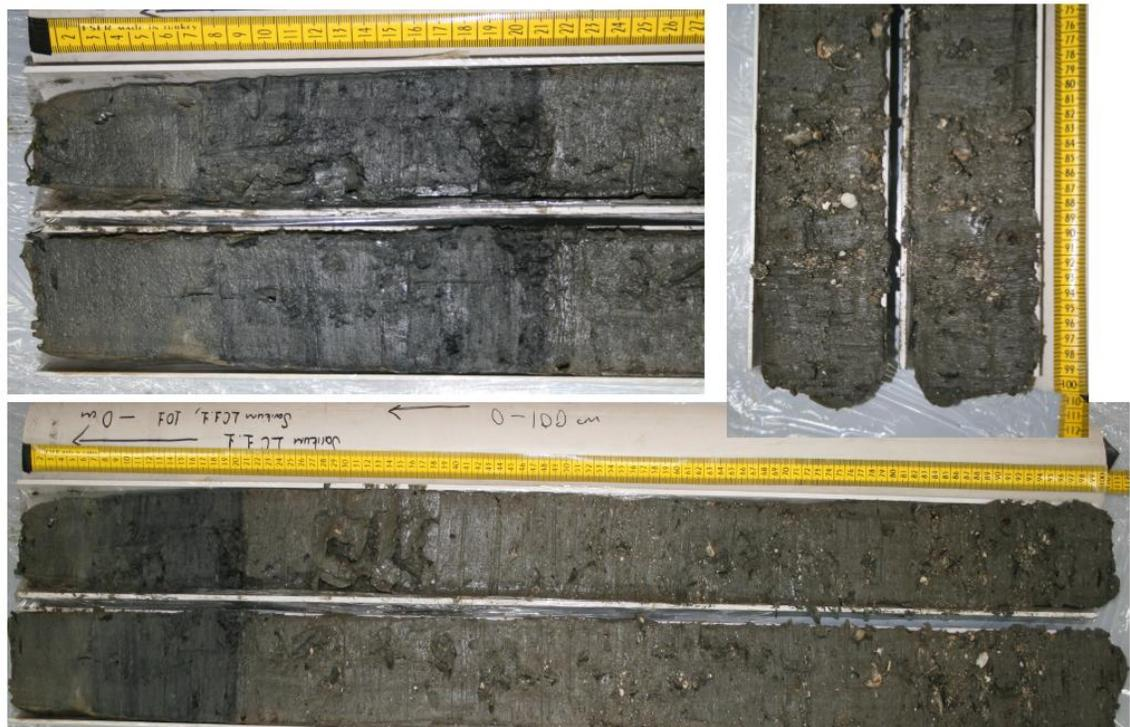
Figure 45. Sarikum Long Core 1 photos. See the transition between SLC1.1 20-21 cm (total depth of 29 cm after splicing with Sarikum Short Core 1) and SLC 2.1 7-8 cm total depth of 16 cm).
