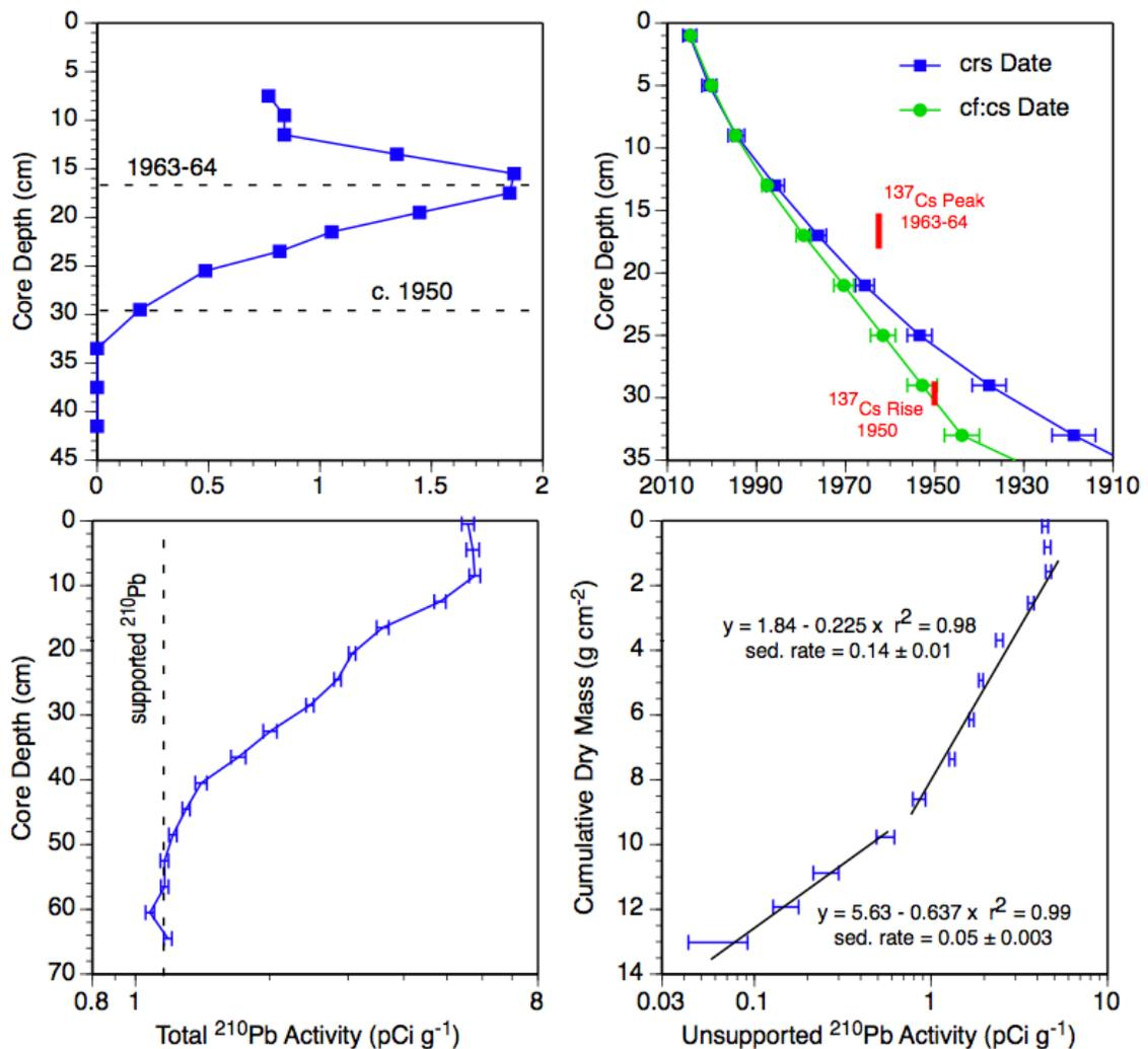
Figure 8.  $^{210}\text{Pb}$  and  $^{137}\text{Cs}$  activity versus depth plots for Terkos Short Core 2 (left), in pCi/g. Depth versus age and dry mass accumulation versus  $^{210}\text{Pb}$  (right) show results of the CRS and CF:CS accumulation models. In this case, the best fit seems to be the CRS model, with an unexplained  $\pm 10$  year error (Doner and Yalçınar, 2006).
