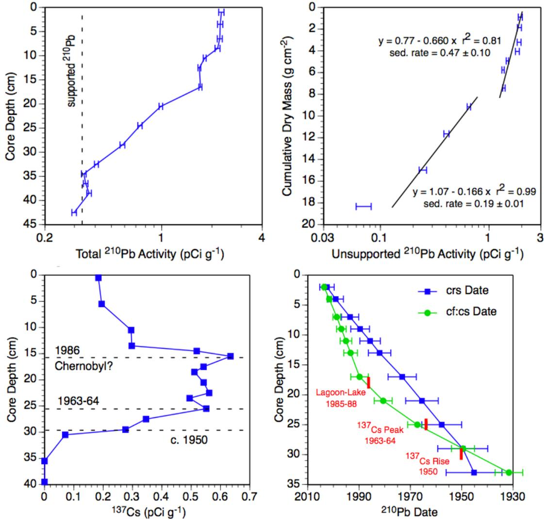
Figure 6.  $^{210}\text{Pb}$  and  $^{137}\text{Cs}$  activity versus depth plots for Büyükçekmece Short Core (left), in  $\text{pCi/g}$ . Depth versus age and dry mass accumulation versus  $^{210}\text{Pb}$  (right) show results of the CRS and CF:CS accumulation models. In this case, the best fit seems to be the CRS model, with an unexplained  $\pm 10$  year error (Doner and Yalçınar, 2006).
