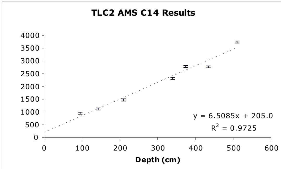
Figure 9. AMS <sup>14</sup>C dating results on 7 bulk sediment samples from Terkos Long Core 2 (BETA Analytic Laboratory). Sedimentation rates are calculated as the inverse value of the slope of the regression line (1 cm/6.5085 yrs).
