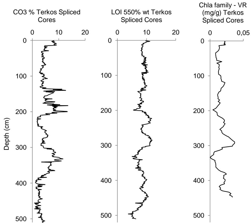
Figure 14. Terkos Spliced Core sedimentary organic matter, carbonate and Chl-a content.
