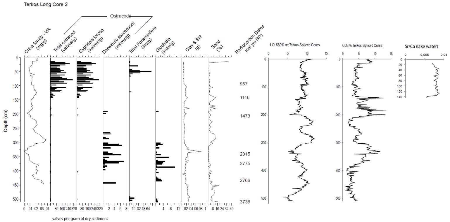
Figure 40. Representation of paleoecological data from Terkos 2 Long and Short Core (combined) ostracoda stratigraphy per g of dry sediment, forams, Glochidia per g, algal production and sand percentage obtained from ostracod analyses and organic and carbonate carbon content.
