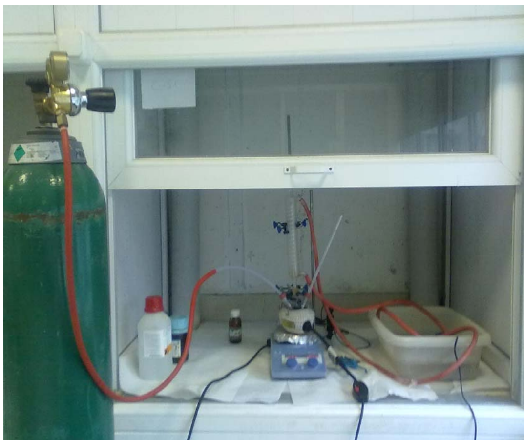
Figure 13 Experimental setup for the synthesis of magnetic iron oxide nanoparticles with Thermal Decomposition Method
