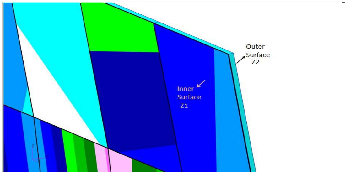
Figure 4.3.3: The layer selection (Z1/Z2) for 2-D skin elements
