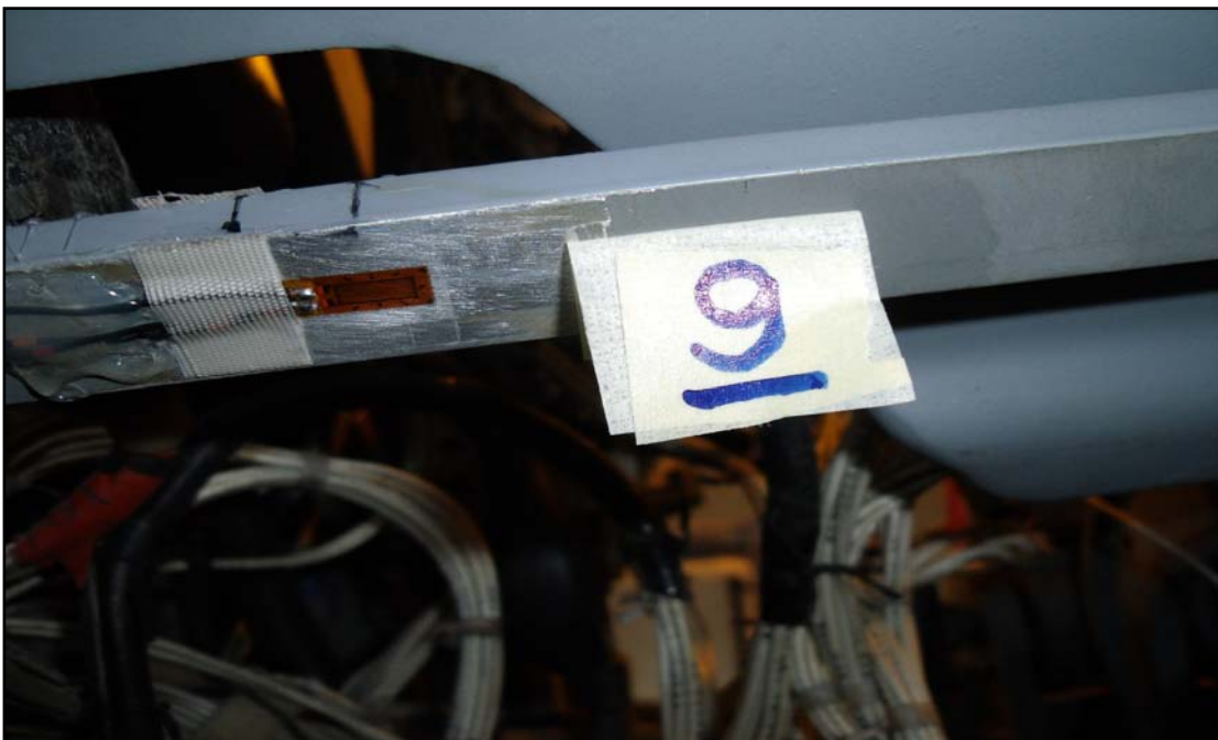
Figure 3.5.7: Linear strain gauge on the tie-bar
