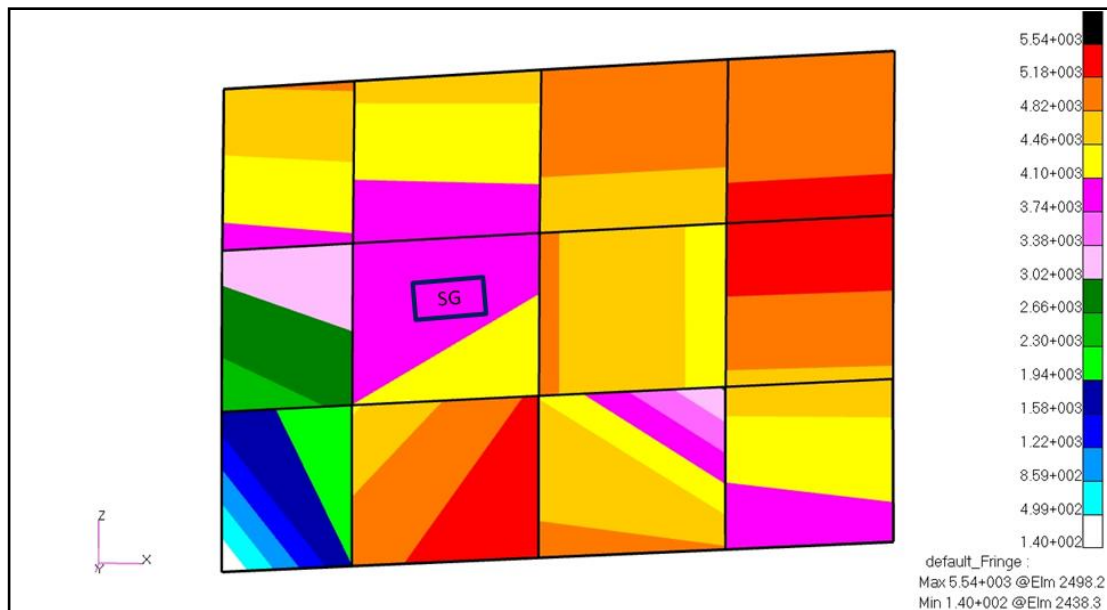
Figure 4.3.2: Stress plot that has no element to element averaging at the nodes.
