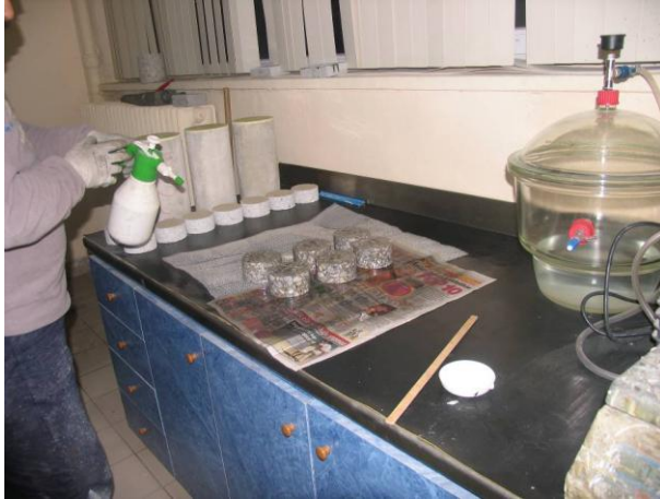
Figure 3.2 Application of coating material 2 to concrete cores
