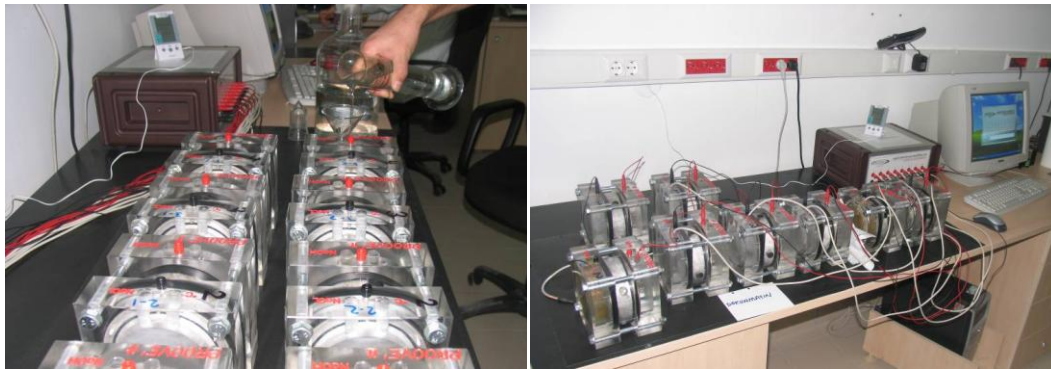
Figure 3.5 a) Conditioning of cores; b) Placement of concrete cores into test cells; c) Placement of solutions; d) Application of electrical potential for chloride ion penetration test phases
