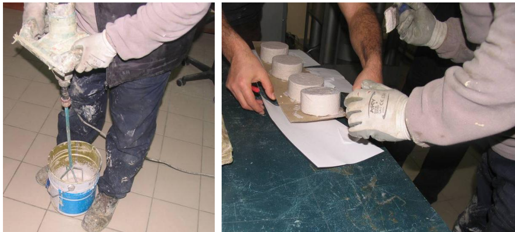
Figure 3.1 a) Preparation of coating material 1; b) application of coating material 1 on concrete cores
