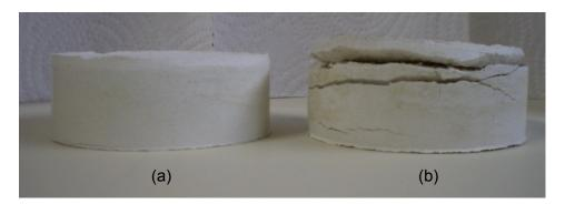
Figure 6.1. Views From 3% lime treated sample after drying ((a)-before first cycle, (b) – before second cycle)
