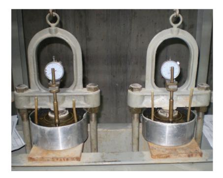
Figure 5.18 View from Oedometers during testing
