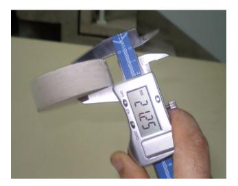
Figure 5.19 Measuring height with digital caliper
