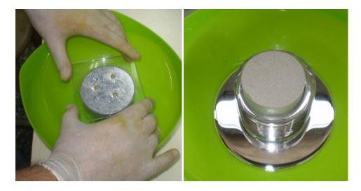
Figure 5.20 Measuring volume with mercury
