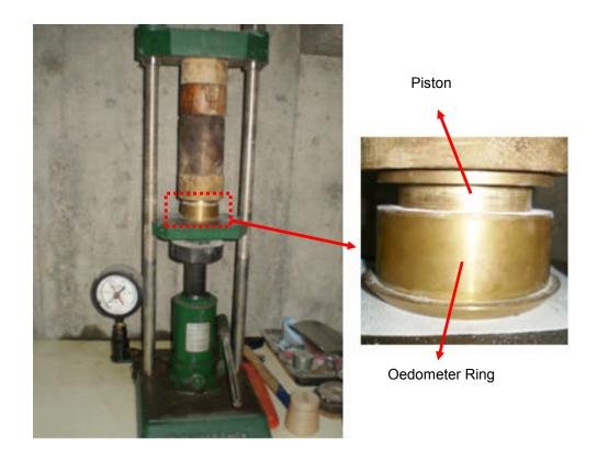
Figure 5.16 A View from Static Compaction
