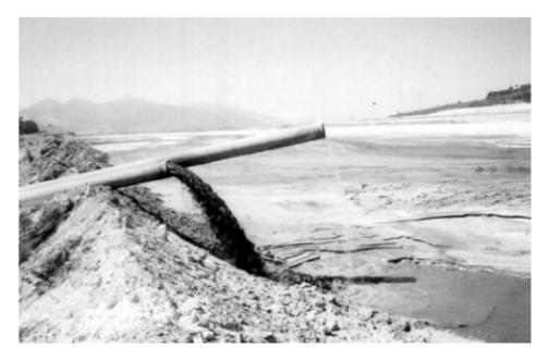
Figure 3.2 Ash Disposal Site of Soma Thermal Power Plant (Baba and Kaya, 2003)
