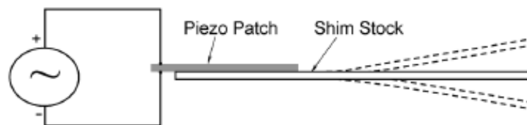
Figure 1.5: Oscillating piezoelectric fan under applied voltages owing to contradiction and expansion of piezoceramic patch.
