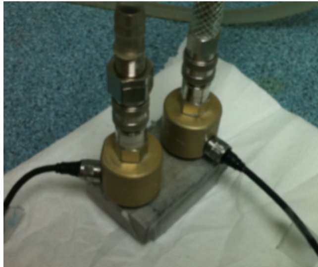
Figure 4.13: Temperature and pressure sensors used to collect data at channel inlet and exit
