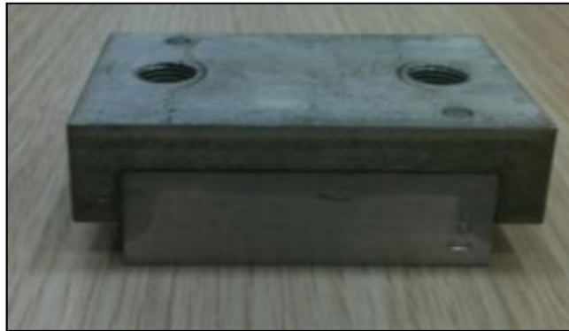
Figure 4.7: Photograph of a brazed channel before finishing
