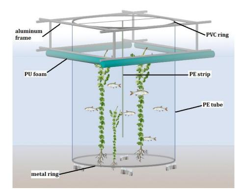
Figure 2: An illustration of the mesocosm setup (taken from Özkan, 2008)
