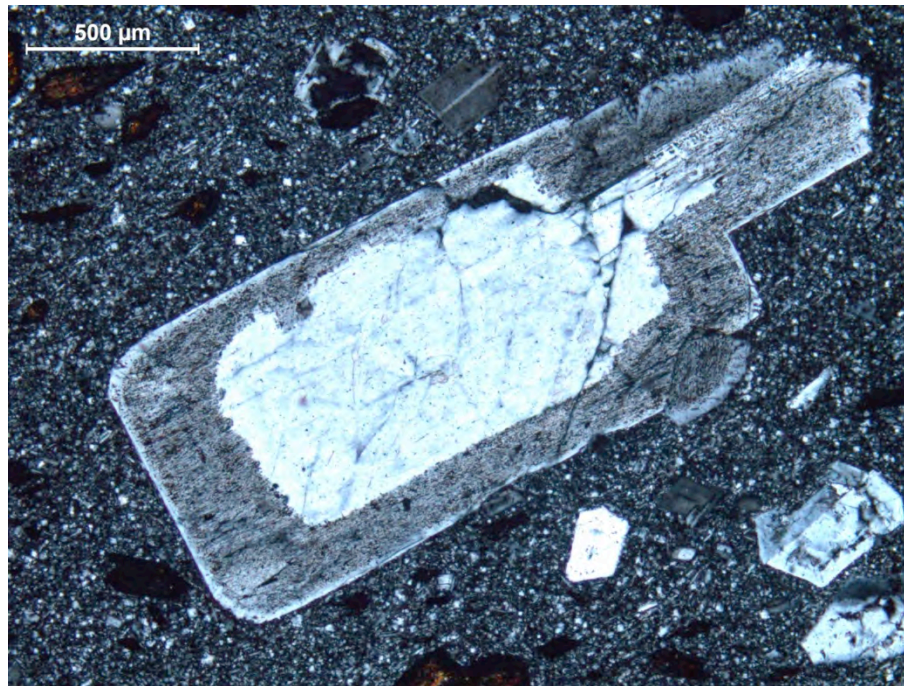
Figure 13 A large plagioclase phenocrystal having sieve texture
