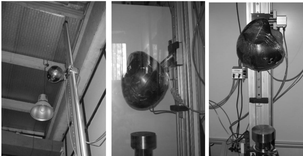
Figure 6.7 General View of the Impact Test Rig for the Helmet Shell
