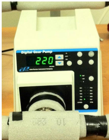
Figure 3: The micro gear pump used in the refrigerant cycle
