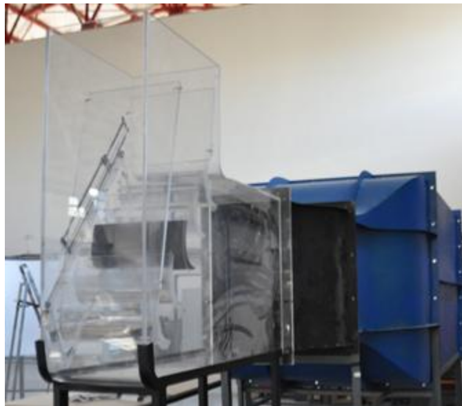
Figure 2.2 Transition duct and transparent test section with the blade row
