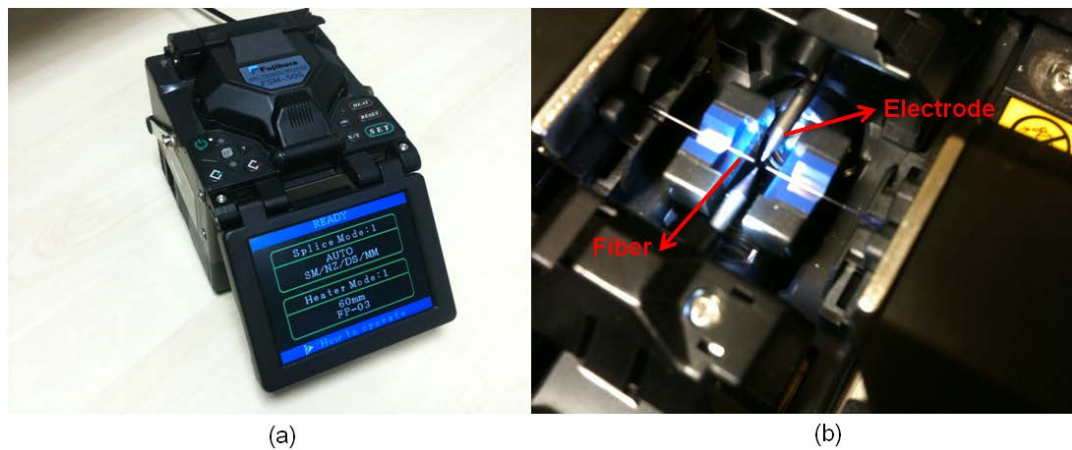
Figure 4-4 (a) Fujikura FSM-50S fusion splicer (b) prepared fibers ready for splicing
