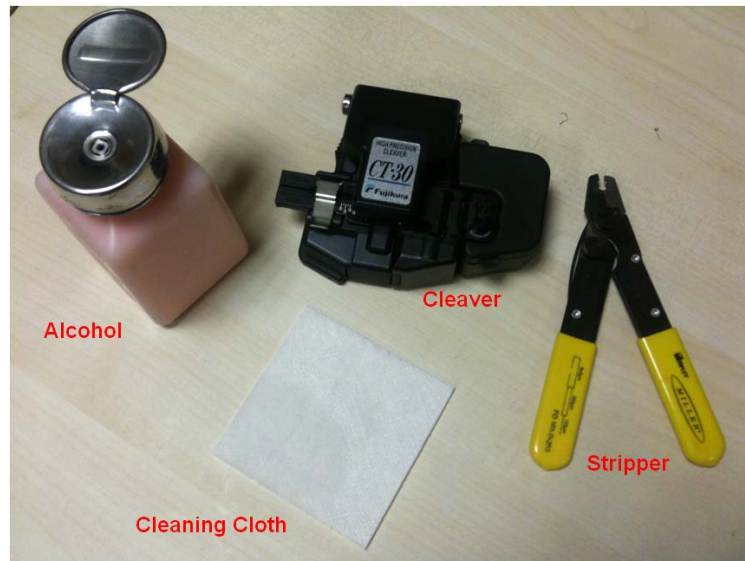
Figure 4-2 Tools necessary to prepare fibers for splicing
