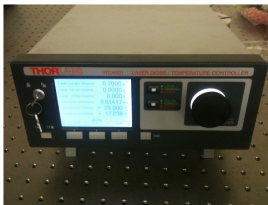
Figure 4-10 Thorlabs ITC4001 laser diode / temperature controller
