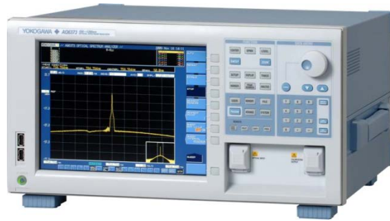
Figure 4-7 Yokogawa AQ6373 optical spectrum analyzer
